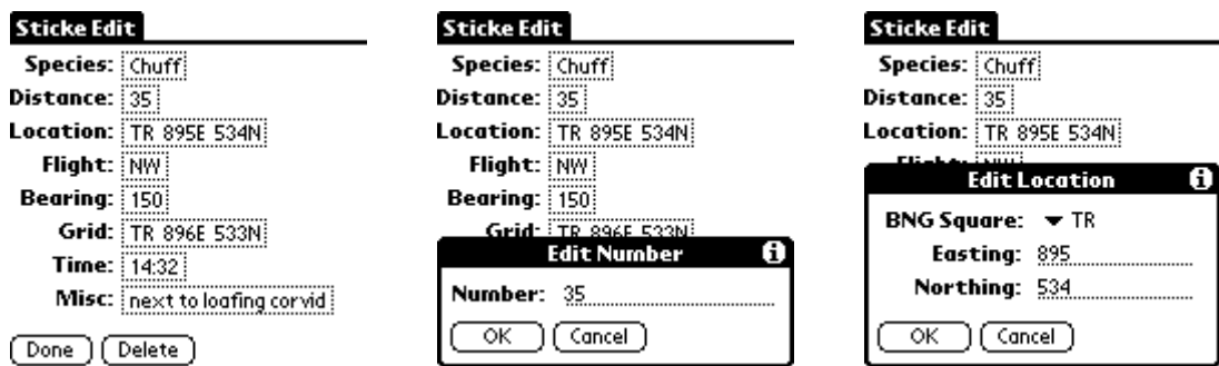
Figure 11. Screen shots of (i) the new stick-e note form display, (ii) manually editing the distance field, and (iii) manually editing the location field.
