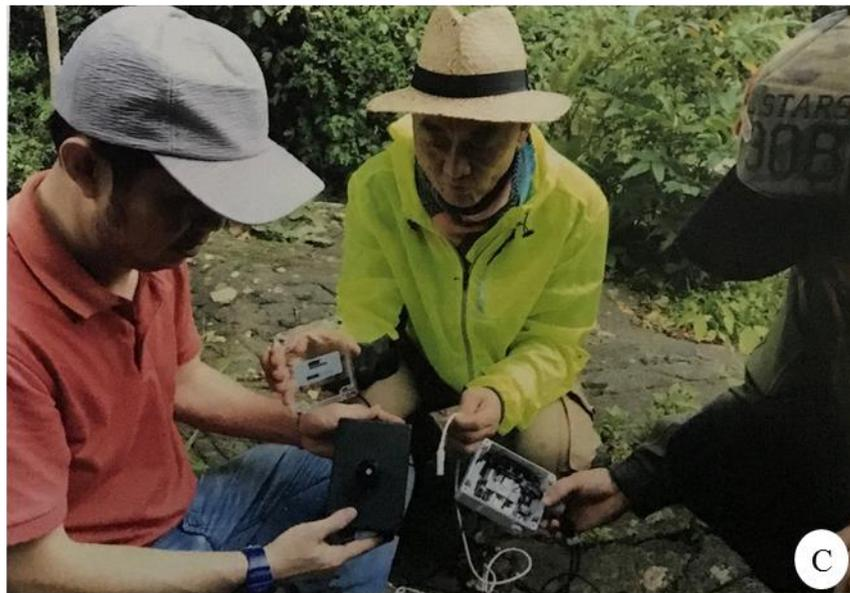
**Appendices Figures 10 (A-C)** Preparing to set up the Hobo Data logger onto the tree trunk in order to measure the moisture, relative humidity, and temperature for fourteen days.
