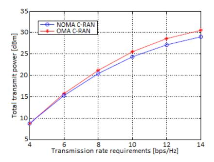
Figure 3.8: Transmit power v.s. minimum transmission rate requirements
