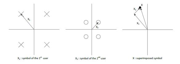
Figure 2.1: SC of two 4-QAM signals [24]
