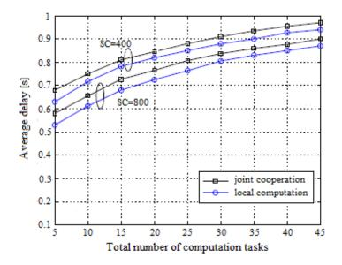
Figure 5.7: Average delay vs the number of computation tasks
