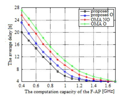
Figure 5.6: Average delay vs the computation capacity of the F-APs
