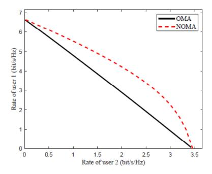
Figure 2.4: The multi-user achievable rate region for downlink NOMA with one BS and two users  $u_1$  is the strong user with  $\frac{|h_1|^2}{\sigma_1^2} = 100$ , while  $u_2$  is the weak user with  $\frac{|h_2|^2}{\sigma_2^2} = 10$ .
