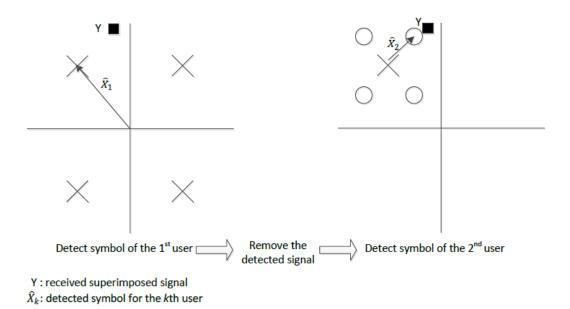
Figure 2.2: SC-SIC detection of two 4-QAM signals [24]
