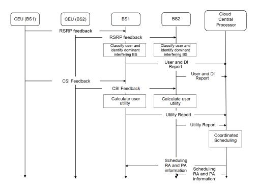
Figure 3.3: Signalling sequences for the proposed approach
