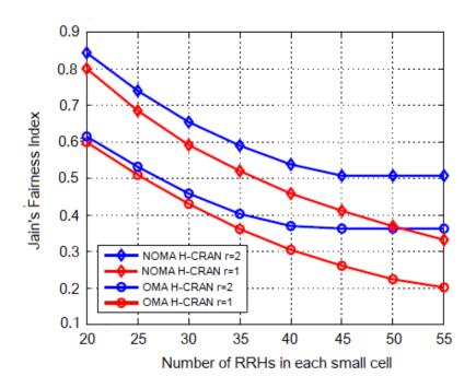
Figure 4.6: Jain's fairness index vs number of RRHs, transmit power at MBS is 43 dBm and the transmit power at RRHs is 29 dBm
