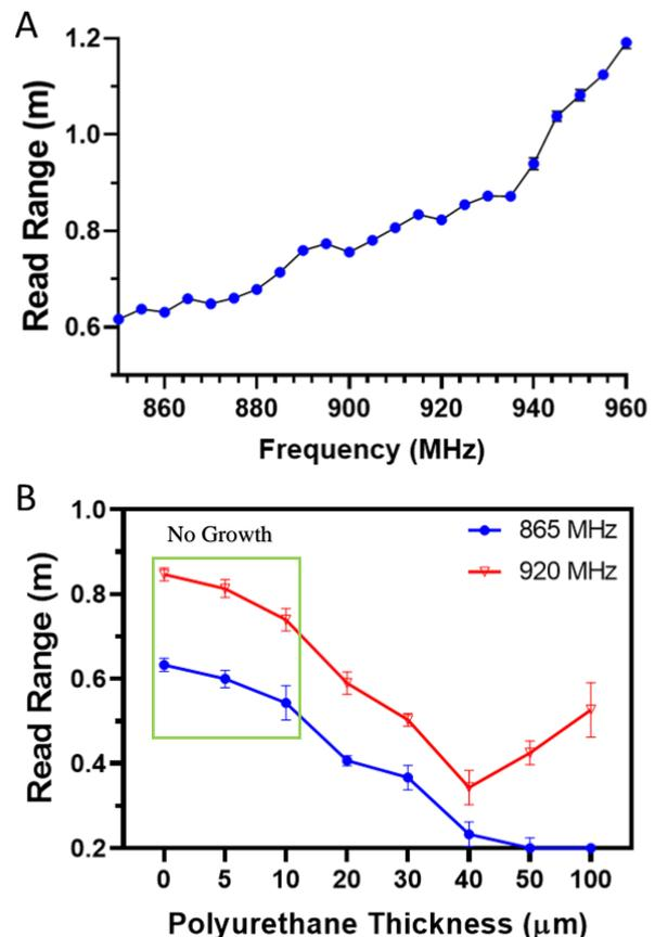
Figure 3 Measurement of sensor function mounted on voice prosthesis within a salt and gelatine neck phantom. A) Antenna measurement over both the EU and USA UHF frequency bands without any biofilm growth adjustments (0  $\mu\text{m}$  polyurethane thickness). B) Sensor function at both the EU (865 MHz) and USA (920 MHz) UHF frequency bands with biofilm layer adjustment to mimic *C. albicans* growth overtime on the voice prosthesis.
