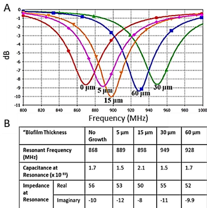
Figure 2 S11 simulated *C. albicans* biofilm growth on the A) antenna sensor and b) simulated matching parameter changes due to increase in biofilm thickness. Till a mature biofilm layer is reached (30  $\mu\text{m}$  thickness), there is a noticeable resonant frequency increase. Once the mature layer thickness doubles in height a top the sensor, there is a reversal in resonant frequency likely due to the saliva decoupling.
