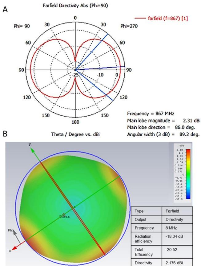
Figure 4 Antenna directivity of a voice prosthesis mounted UHF RFID convoluted antenna sensor within a gelatine phantom. A) The polar plot showed a 2.31 main lobe magnitude visualized with a phi 90° cut. B) The total efficiency and antenna directivity shown in a 3D model view.
