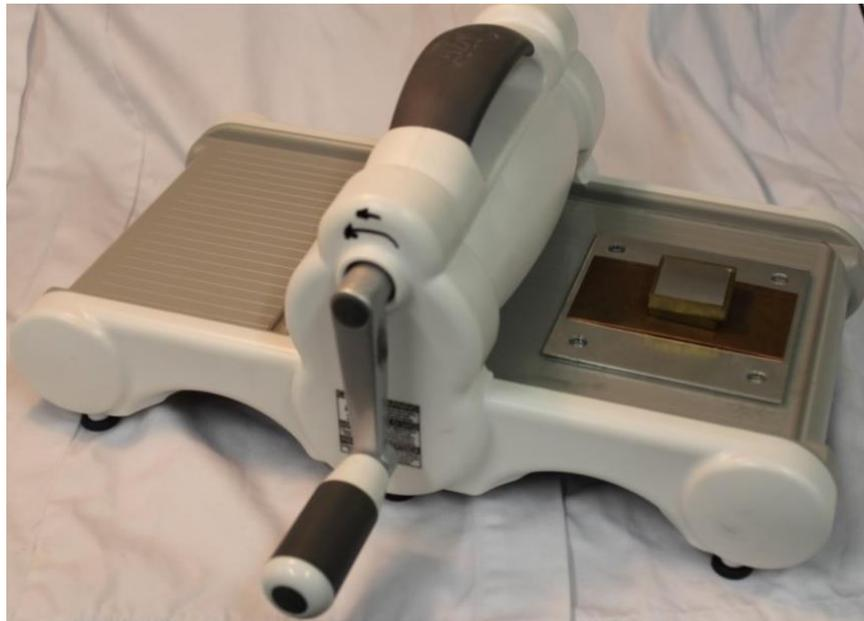
Figure 3.23: The prototype punch being used to punch a 100 micron thick aluminium foil electronic burst disk on a "Sizzex Big Shot" die cutting machine.
