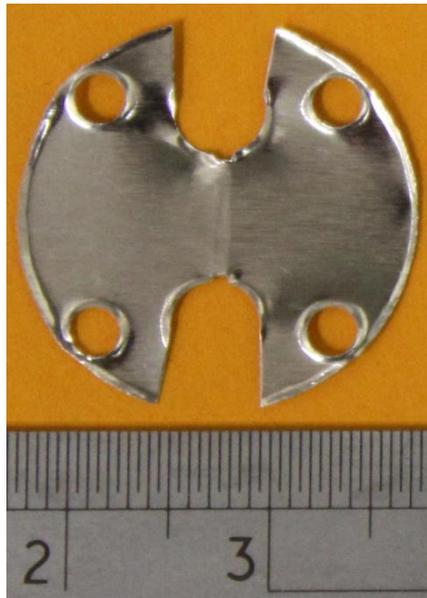
Figure 3.34: An electronic burst disk foil layer with the notches cut (scale divisions are 0.5 mm).
