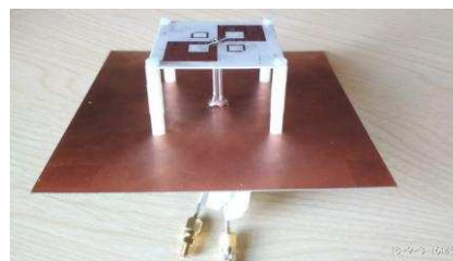
Fig. 14. Photograph of the fabricated prototype of the proposed dual-polarized antenna.
