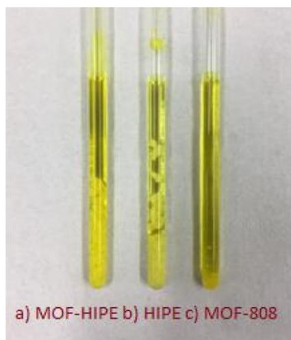
**Figure 5.4.** An image highlighting the difference in dispersion of MOF-808. Both tube a) and c) contain the same quantity of MOF. Tube b) contains no MOF-808. Tube a) shows the superior dispersion provided by the HIPE polymer matrix.
