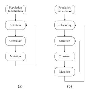
Figure 1. Introducing a refactoring step into genetic programming. In (a) the traditional GP steps; (b) the GP steps with the addition of a refactoring step.
