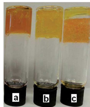
Fig. 4 Organogels containing (a) 3 (9.6 mg), DMSO (0.8 mL), DCP (0.01 mL), 6 (80 mg); (b) 3 (9.6 mg), DMSO (0.8 mL), DCP (0.05 mL), 6 (80 mg); (c) 3 (9.6 mg), DMSO (0.8 mL), DCP (0.10 mL), 6 (80 mg).
