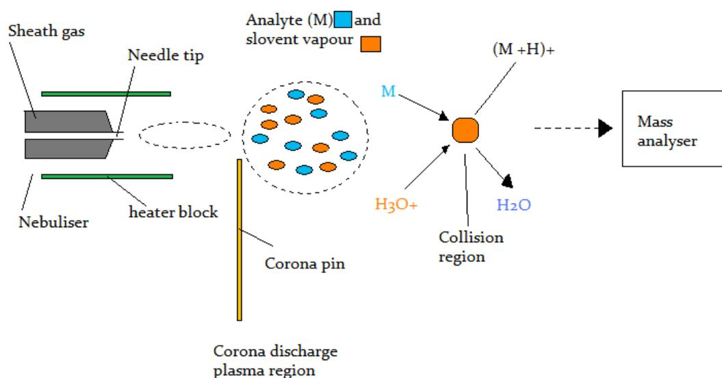
Figure 10: APCI schematic showing the main components and how ions are formed. Image replicated by Tom Cull from <http://www.chm.bris.ac.uk/ms/apci-ionisation.xhtml> viewed on 25/09/2018.
