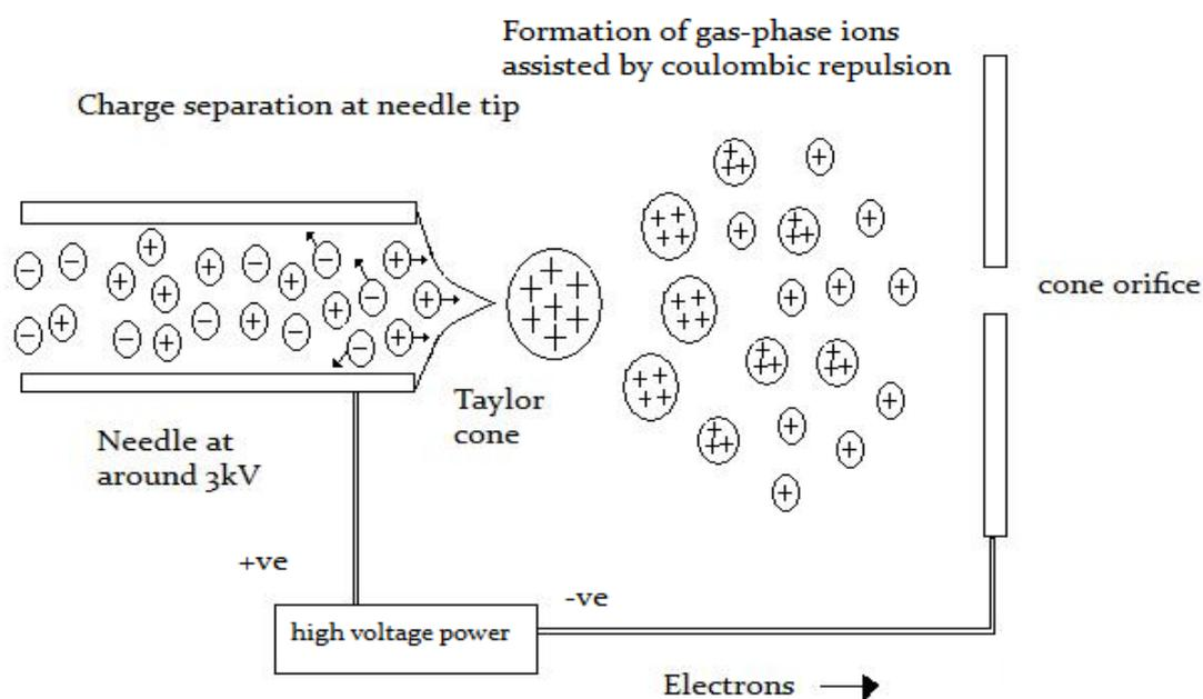
Figure 9: ESI schematic showing the main components and sample conversion into ions including the Taylor cone and the Coulomb explosion. Image drawn by Tom Cull, replicated from D. Watson, in Clarke's Analytical Forensic Toxicology, ed. S. Jickells and A. Negrusz <sup>35</sup>.
