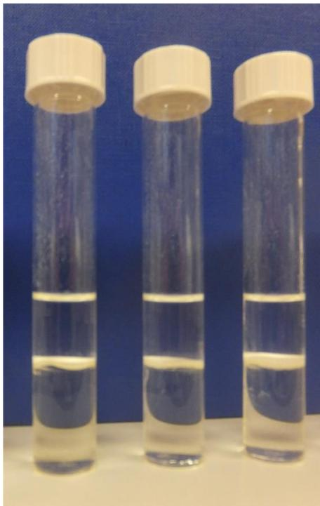
*Figure 19: 10 mL glass tubes after centrifugation at 3000 rpm for 10 minutes. Two layers are clearly defined layers with a protein disc sandwiched between the two. Refer to comment in declaration regarding photographs.*
