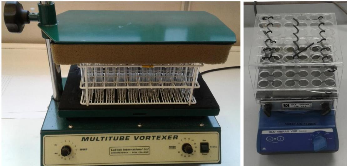
*Figure 32: Comparison images of a Lab-tek international vortexer and a IKA VIBRAX VXR vibramixer. Refer to comment in declaration regarding photographs.*
