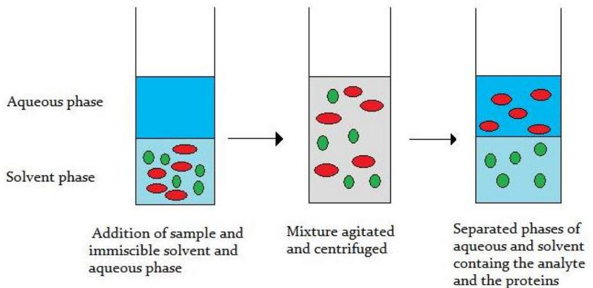
Figure 12: Schematic of the LLE extraction process
