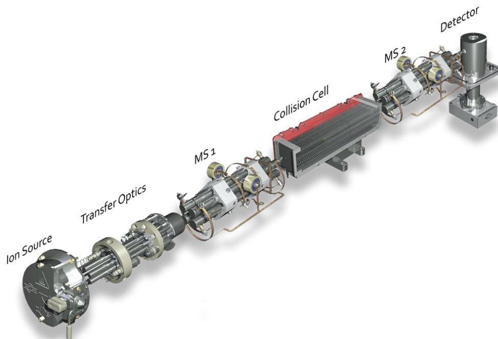
Figure 7: Schematic diagrams of tandem mass spectrometry indicating the individual components. Image belongs to Waters, Manchester, but given permission to use in this thesis.
