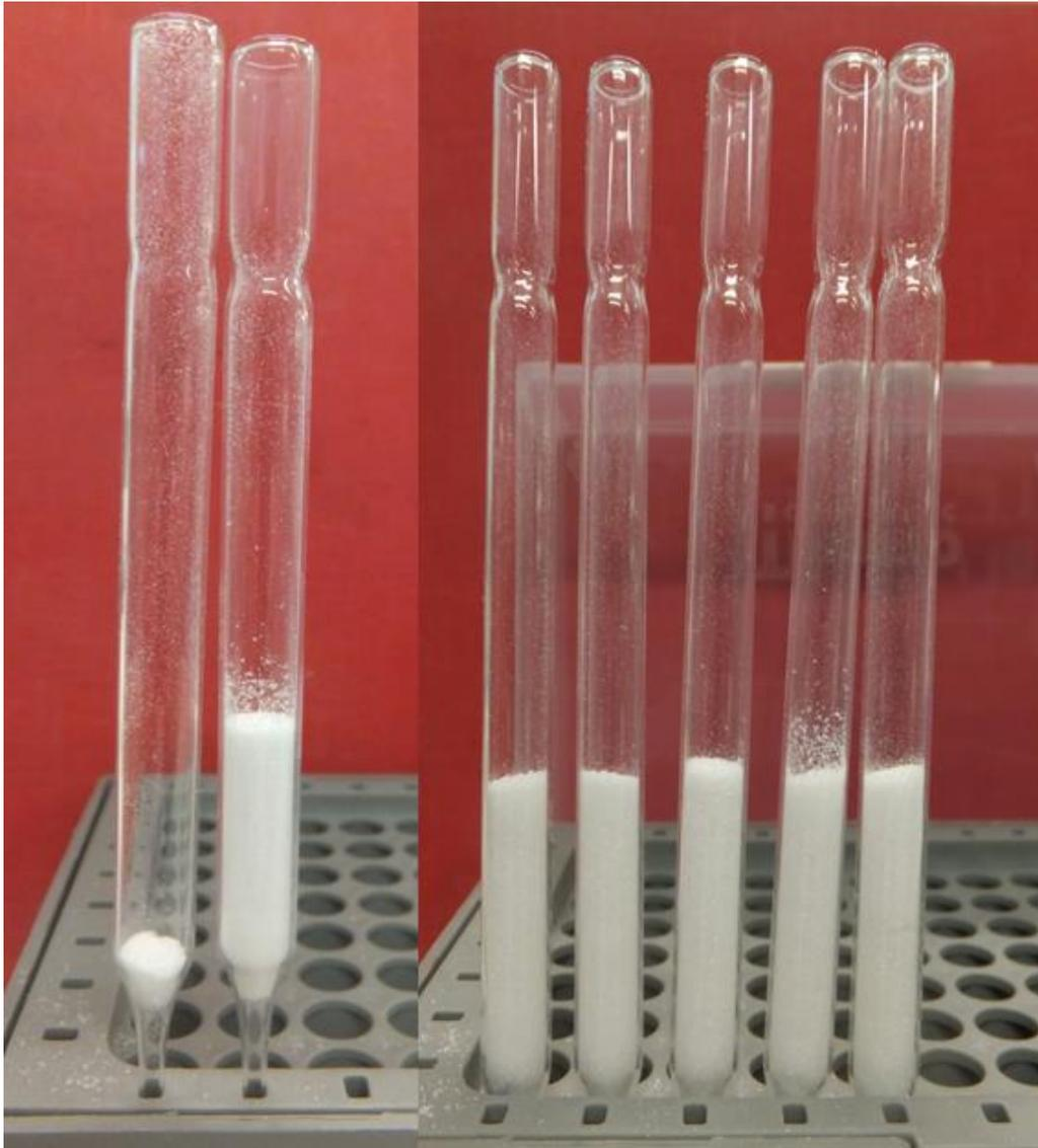
*Figure 16: Sodium sulphate columns. Image on right shows column with cotton wool bung and wool with sodium sulphate. Image on left shows prepared columns. Refer to comment in declaration regarding photographs.*
