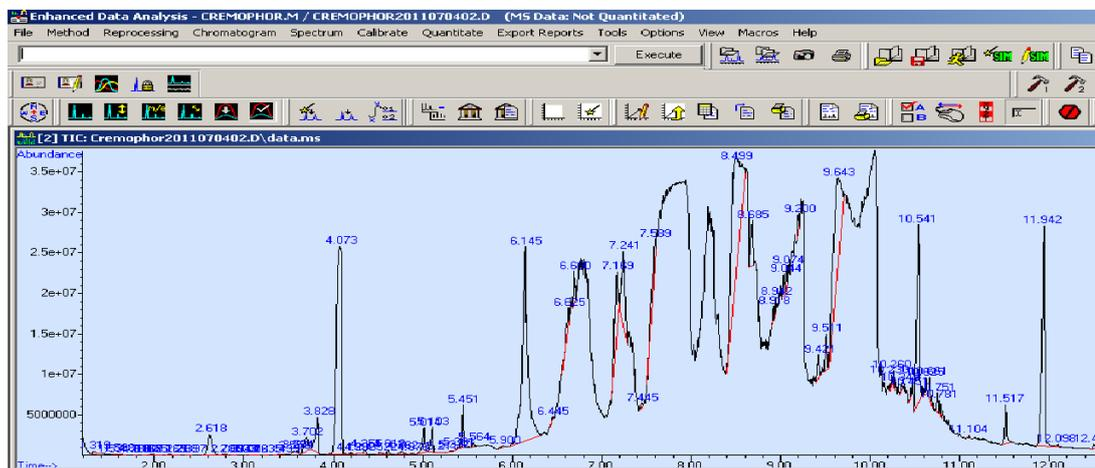
Figure 23: Image showing the GC-MS spectrum produced after the injection of an extracted CrEL standard. Peaks such as these occurred when the column began to saturate and eventually block.
