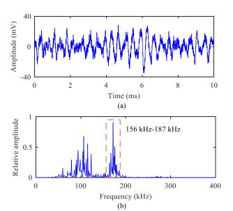
Fig. 9. Typical signal waveform and its corresponding PSD. (a) Time domain. (b) Frequency domain.
