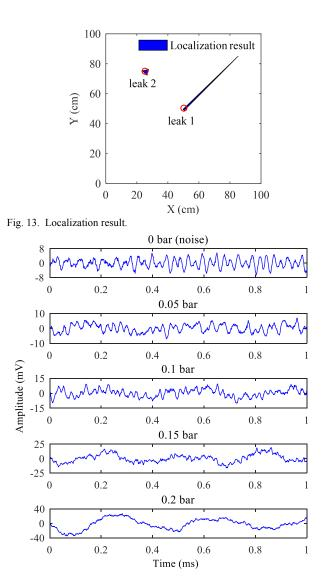
Fig. 14. AE signals corresponding to different leak pressures.
