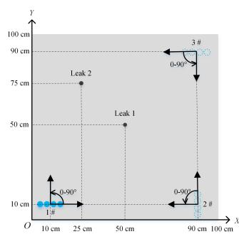
Fig. 6. Arrangement of the sensor array.
