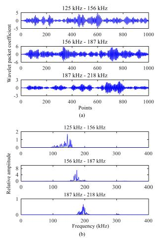
Fig. 10. Wavelet packet coefficient and PSD corresponding to several nodes. (a) Wavelet packet coefficient. (b) PSD.
