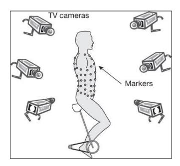
Figure 2.7 Optoelectronic plethysmography: principle of measurement (Vogiatzis et al., 2005)
