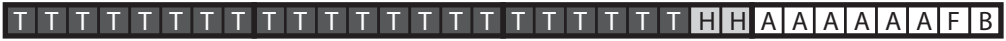
Fig. 3. Jikes RVM object status word bits: thin lock (T), hash state (H), unused bits available (A) for use by the GC, forwarded (F) and busy bits (B).
