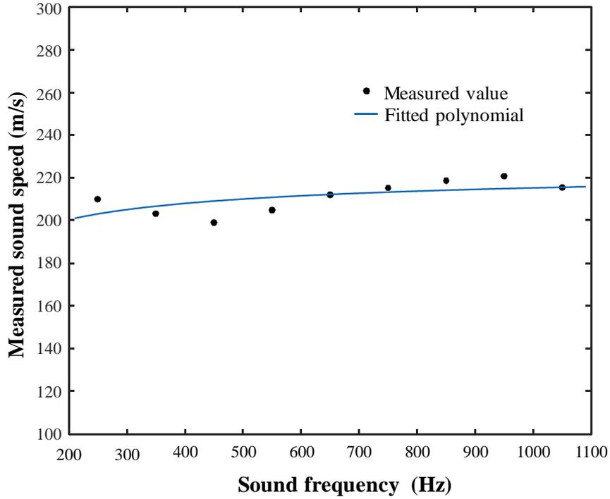
**Figure 11.** Measured sound speed under different sound frequencies
