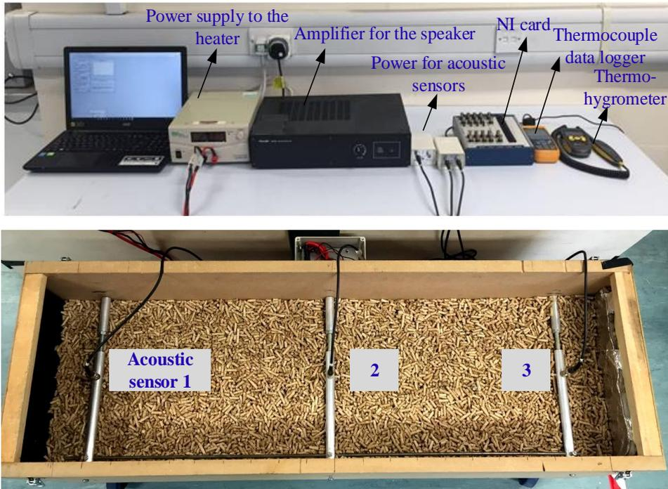
**Figure 6.** Experimental setup of biomass temperature measurement system
