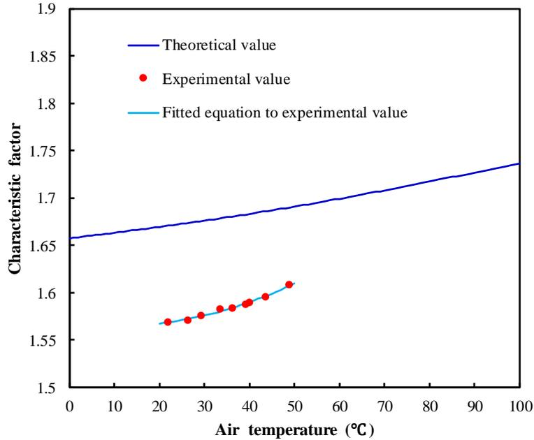
**Figure 12.** Relationship between characteristic factor and temperature
