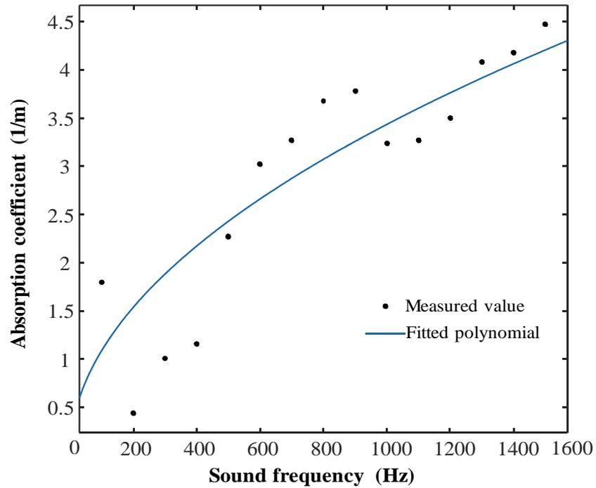
**Figure 10.** Sound absorption coefficient under different sound frequencies
