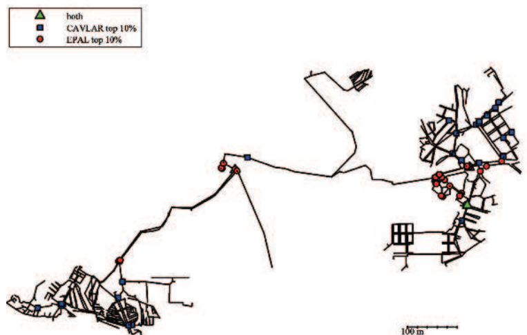
Figure 5 Top 10% important valves according to EPAL ranking and CAVLAR CML ranking
