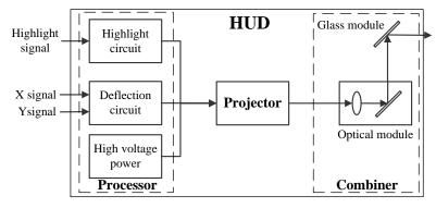
Fig. 3. The structure of HUD system [33].
