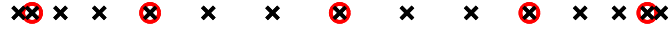
Figure 1: Circles show Chebyshev points of the first kind for n = 5 and crosses for n = 15 .
