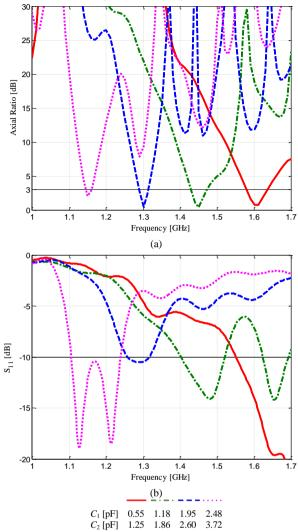
Fig. 5. Illustration of tuning capability (a) AR (b) reflection coefficients
