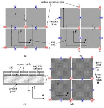
Fig. 1. Unit cells of the dual polarized active AG structure with varactors and resistors. (a) upper layer (b) lower layer (c) magnified cross-sectional view (d) alignment of the upper and lower layers
