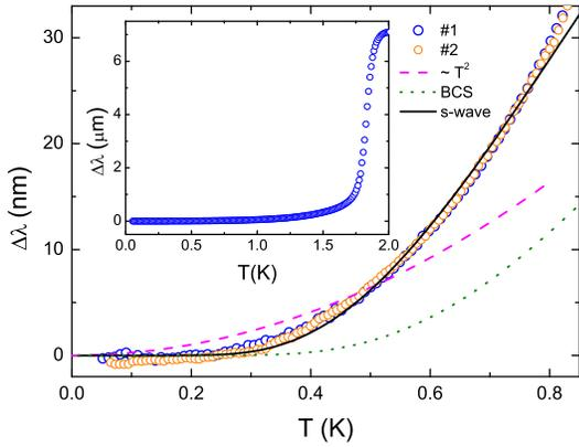
FIG. 1: (Color online) London penetration depth  $\Delta\lambda(T)$  of two samples of LaNiGa<sub>2</sub> at low temperatures. The solid and dashed lines show fits of  $\Delta\lambda(T)$  to an  $s$  wave model with  $\Delta(0) = 1.30k_B T_c$ , and a  $T^2$  dependence respectively. The dotted line shows  $\Delta\lambda(T)$  for an isotropic, weakly coupled BCS superconductor. The inset shows  $\Delta\lambda(T)$  for sample #1 up to 2 K.
