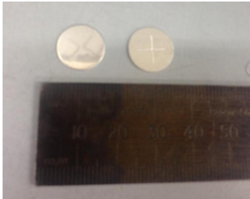
Figure 8: Image showing two aluminium burst discs. The disc is broken once a desired pressure is realised within the pump tube. The discs are 12.7 mm in diameter and 0.5 mm thick.
