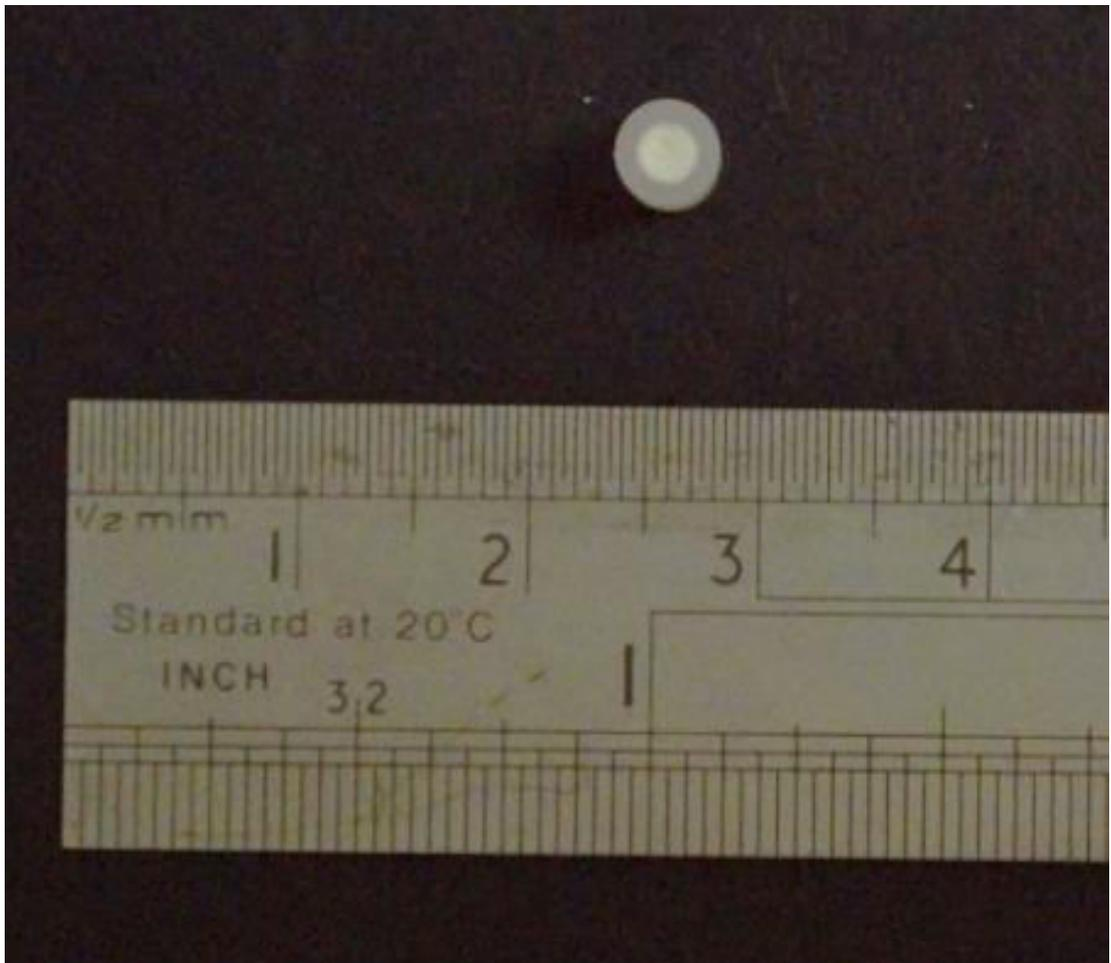
Figure 20: Top down view of the nylon sabot showing the well containing the diatomaceous soil. This well is 2.55 mm in diameter and 2.5 mm in depth.
