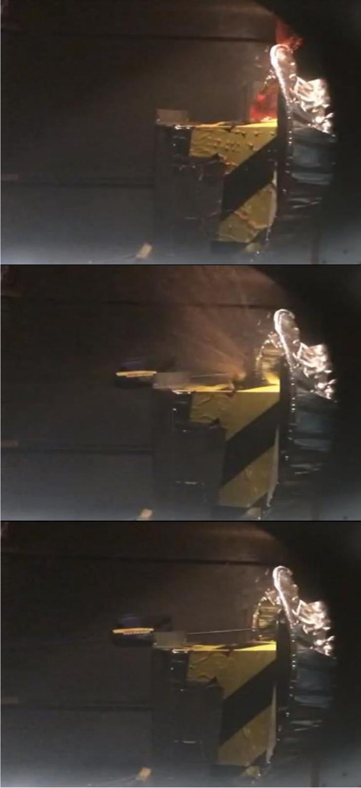
Figure 56: A sequence of 3 images showing the impact of the second shot featuring the counter-bored sabot with an inset lid at a velocity of  $0.897 \text{ km s}^{-1}$ . The sabot enters the target box via an aperture which is covered by a thin plastic lining. The box had been pre-filled with red dyed water which can be seen emerging in the second and third frame in this sequence.
