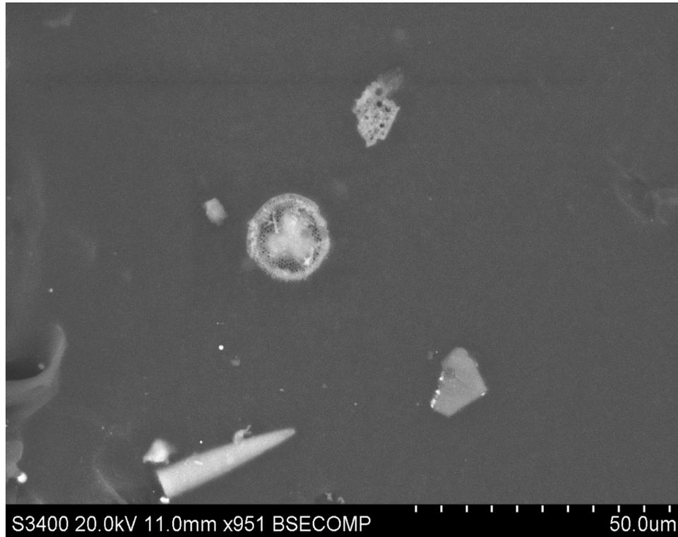
Figure 43: This image shows an intact microfossil in during a general inspection of the SEM stub, containing filtrate following the shot at  $2.05 \text{ km s}^{-1}$ . No intact fragments were found during an SEM map.
