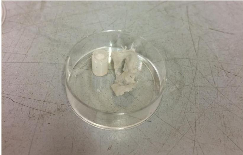
Figure 61: Intact sabot containing diatomaceous soil in suspension (right) before a shot. (Left) the new sabot design following the  $2.17 \text{ km s}^{-1}$ , the sabot has significantly deformed but was capable of transmitting its contents into the target.
