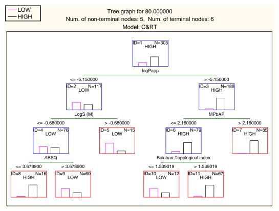
**Figure A3. 15**. Model 8; C&RT permeability experimental solubility (logS M) and melting point based absorption potential (MPbAP) model when higher misclassification costs of two were applied to the high MPbAP node only
