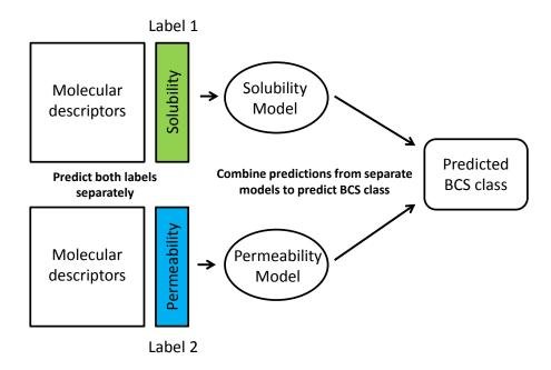
**Figure 5.1**. How the binary relevance problem transformation method works for BCS class prediction
