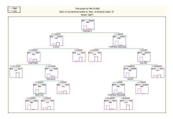
**Figure 8.2.** Tree graph for C&RT analysis using random forest predictor importance as feature selection method with equal misclassification costs applied to preprocessing C&RT (Model 2 in Table 8.3)
