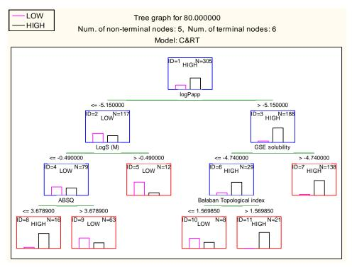
**Figure A3. 17.** Model 10; C&RT permeability, experimental solubility (logS M) and predicted solubility (GSE) model when higher misclassification costs of two to reduce false positives were applied to high GSE solubility node only
