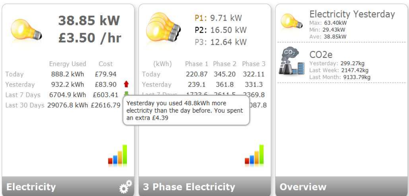
Figure 13. Real time indication of savings and wastages (red and green arrows).
