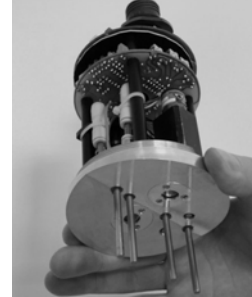
Fig.4 Combined particle sizing and flow metering sensor
