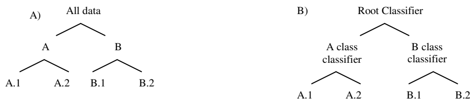
Figure 1: Example of a hierarchical dataset (a) and how that hierarchy may be reflected in a tree of classifiers (b) ready for a top-down approach to classification.
