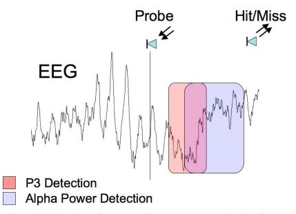
Figure 4. Detection of acknowledgement signals in the data from a single example trial. The time of the probe input corresponds to the onset of the visual stimulus, and the following two analyses are performed, producing a hit or miss output.
