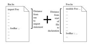
FIGURE 1.2. Measuring distance across module boundaries.
