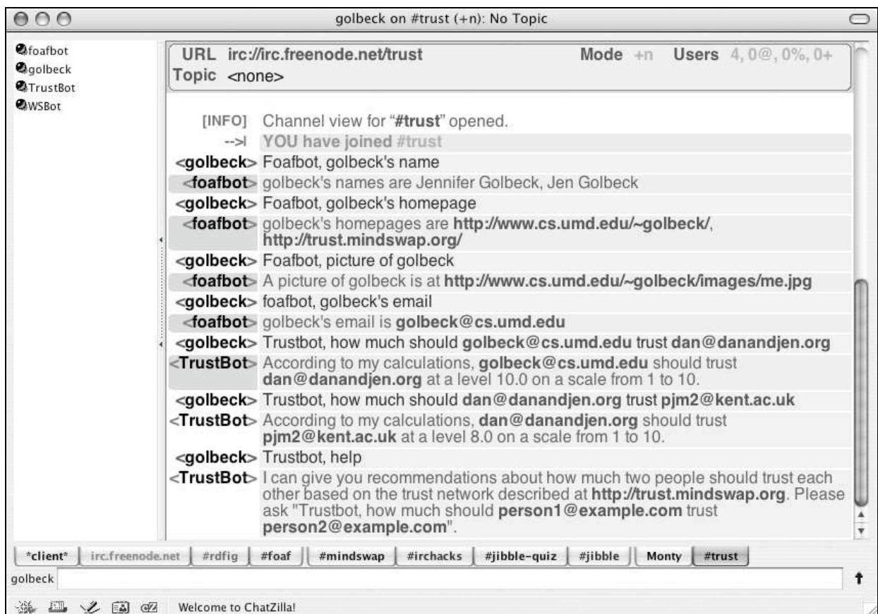
Figure 2: interactions between user (golbeck) and bots (TrustBot and foafbot). Both bots maintain a model built from Semantic Web data and use the IRC interface for receiving queries to those models.
