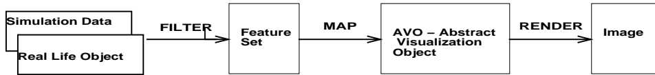
Figure 1: Dataflow model. The data is filtered , to create a subset, which is then mapped into a representation which can be displayed
