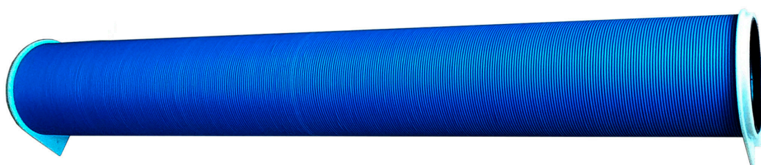
Figure 11. Large solenoid used for verification of sensitivity.
