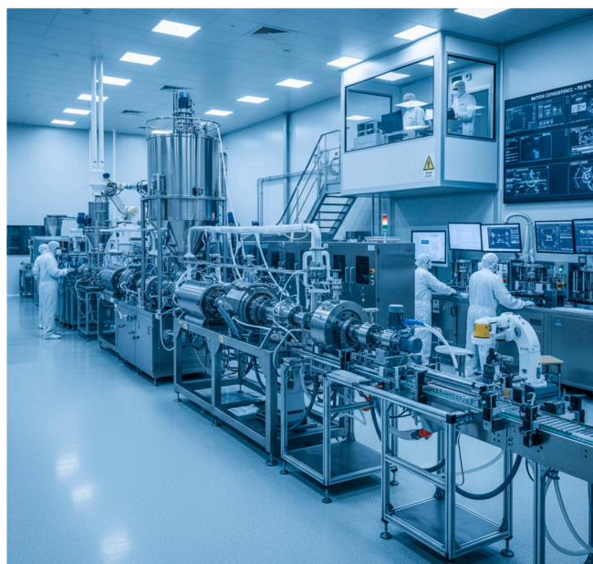
Fig. 12. A continuous HME line at industrial scale.
