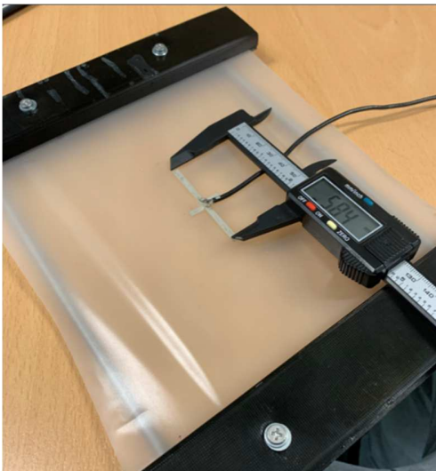
Fig. 9. Antenna sensor being stretched in the Y direction.
