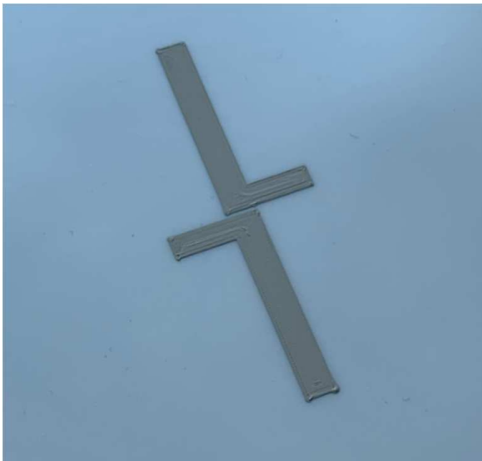
Fig. 8. Printed stretched antenna sensor.
