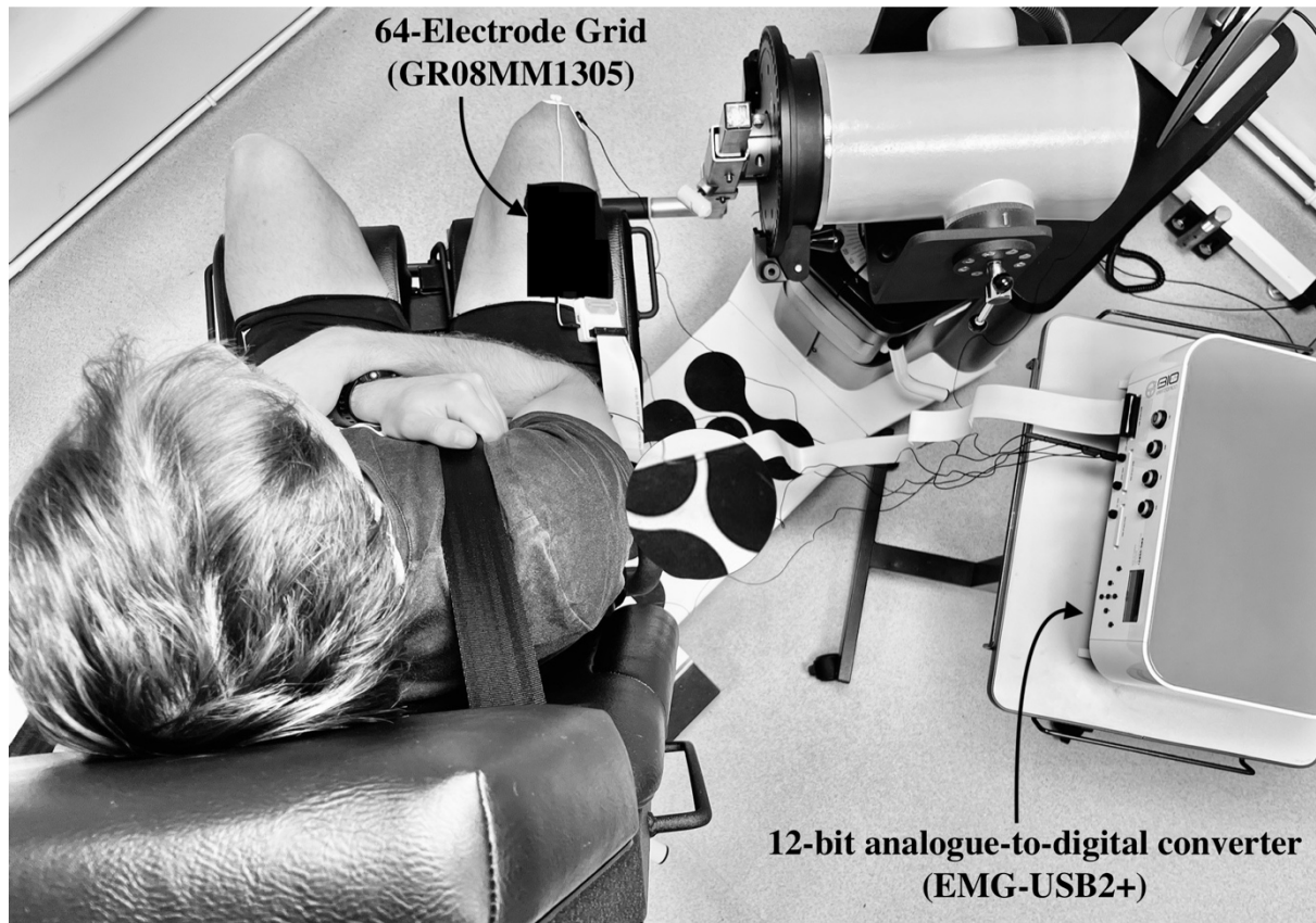
Figure 3.6. HD sEMG 12-bit analogue-to-digital converter (EMG-USB2+, 64-channel EMG amplifier; OT Bioelettronica, Torino, Italy) and isokinetic dynamometer (Cybex HUMAC Norm; CSMi, Stoughton, MA, USA) set up for the recording of interference EMG signals from the participants vastus lateralis muscle of the right leg during isometric knee extension contractions using semi-disposable 64-electrode grids (5 rows x 13 columns; 4 mm electrode diameter; 8 mm interelectrode distance; GR08MM1305; OT Bioelettronica, Torino, Italy) secured with kinesiology tape (Kinesio Precut, Albuquerque, NM, USA).
