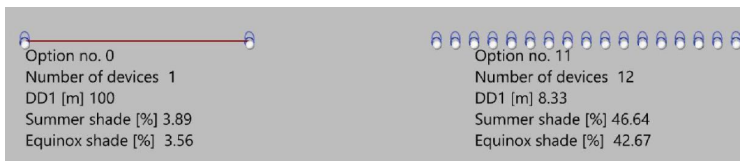
Figure 6.23 Visualisation of the shading devices configuration (sample of two configurations). For each scenario, in addition to the devices and the resulting shadows, a brief description of input parameters and resulting DD_1 and shaded length is provided [TH].
