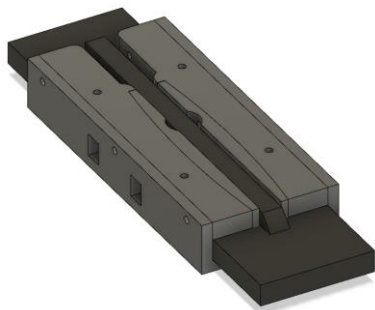
Figure 42 - Exoskeleton Hardpoint slots (Pre-existing Orthosis in black)
