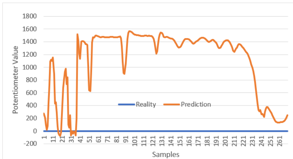
Figure 77 - Prediction System trained only on walking data knee angles struggles to predict the wearer's knee angle standing still, as it has not been trained to "know" what standing still is. 20Hz Sampling Rate.
