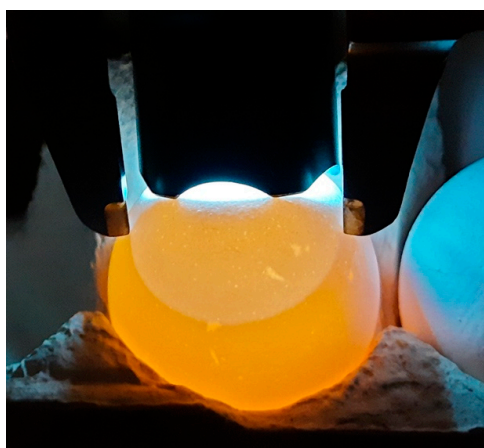
Figure 5. Measuring the diameter of the egg air cell using a caliper [173].
