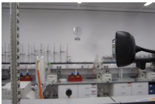
Figure 7: Using webcams to enhance visual feedback. A webcam is clamped on a retort stand such that it can view a burette. The webcam image will be magnified on to a screen (not shown in the image) such that it will allow a student with visual impairment to better see the start and end points of the titration. Also, the burette, which is clamped to a retort stand, is placed inside a large spill tray.
