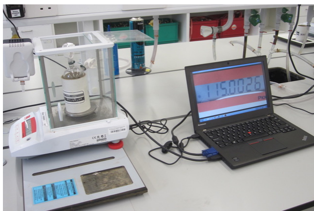
Figure 12: Magnifying readings. Image shows how the digital readout of a weighing scale can be captured by a webcam and displayed on a laptop with the image magnified to improve its readability. It also allows a student to get close to the screen without impediment, to better read the digits.
