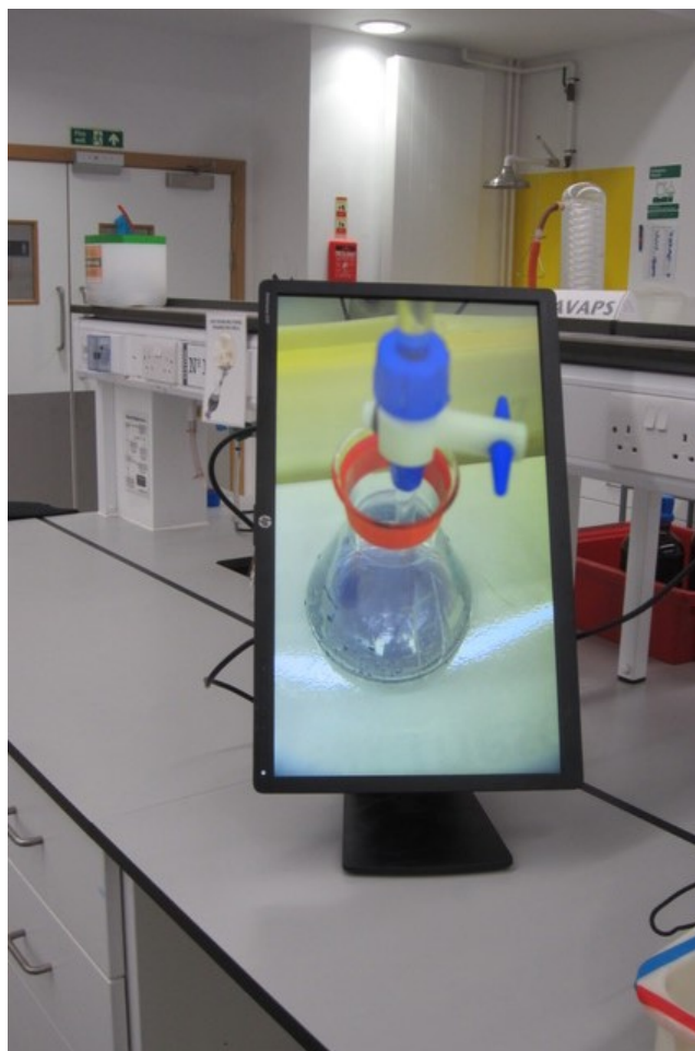
Figure 10: Webcam display. Image of the titre flask captured by a webcam and displayed on a screen allowing the student to observe the endpoint of the reaction without needing to get close to the flask and chemicals.
