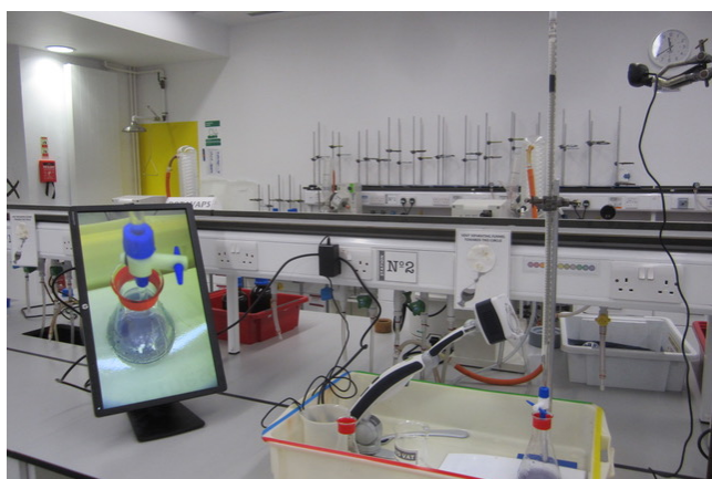
Figure 9: End-point visualization. A webcam is focused on the burette, set-up inside a splash tray, to visualise the burette reading. A separate webcam is focused on the titre flask to observe the endpoint. To the left of the splash tray is a screen showing the titre flask magnified for better visualisation. This also means that the student does not have to get close to the chemicals in the flask.
