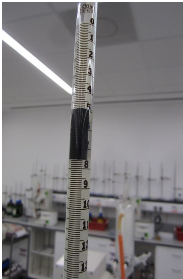
Figure 8: Contrast on the burette. The burette has black tape applied in the critical area where a reading will occur. This is to allow for better visual contrast between the tape and meniscus of the solution.
