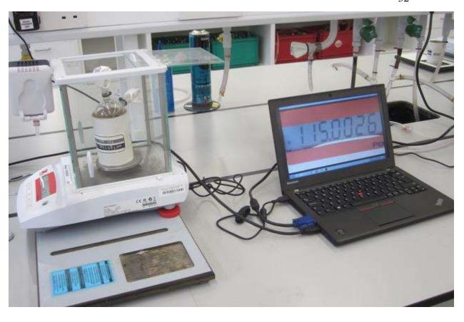
Figure 12 Magnifying readings. Image shows how the digital readout of a weighing scale can be captured by a webcam and displayed on a laptop with the image magnified to improve its readability. It also allows a student to get close to the screen without impediment, to better read the digits.
