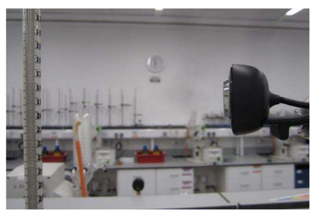
Figure 7 Using webcams to enhance visual feedback. A webcam is clamped on a retort stand such that it can view a burette. The webcam image will be magnified on to a screen (not shown in the image) such that it will allow a student with visual impairment to better see the start and end points of the titration. Also, the burette, which is clamped to a retort stand, is placed inside a large spill tray.
