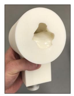
*Figure 5.6.* Anatomical Throat Model internally coated with 'wet' ethanolic Brij®35 and glycerol solution.
