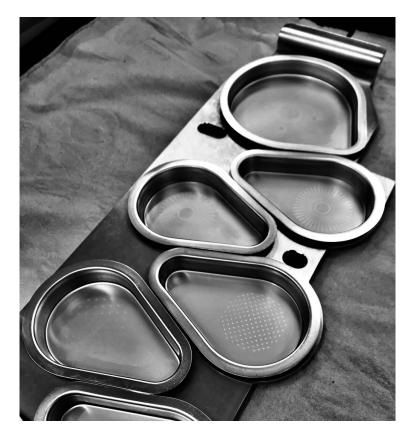
**Figure 5.8**. NGI collection plate stages [four to eight] with beclomethasone dipropionate (BDP) deposited from Qvar ( $00 \mu g$  at 100 L/min. (black and white image with contrast filter applied for better visualisation of the fine particles deposited).
