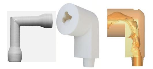
*Figure 5.5.* United States Pharmacopeia throat model [left]. Emmace Consulting anatomical throat model (medium) [middle]. Interior surfaces of Emmace Consulting anatomical throat model [right].
