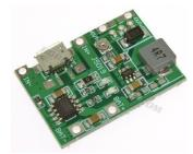
FIGURE 4.7: LiPo battery charger used to recharge the lithium-ion battery.
