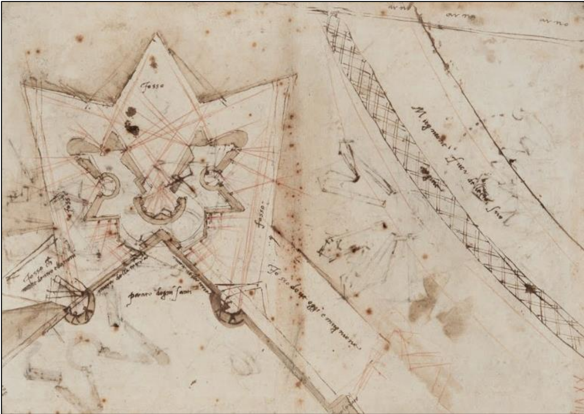
Fig. 7 A military map showing how the architecture of this star fort is deployed to allow the best advantage of return fire. This example is by Michelangelo for the fortification of Florence in the 1520s, Wikimedia Commons public domain.
