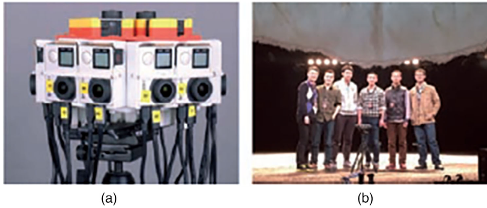
FIGURE 12 A setup for acquiring and broadcasting live VR, (a) dual panoramic camera array (DPCA), and (b) live broadcasting of 360° 3D VR [25].
