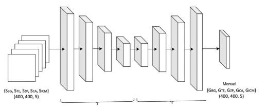
Encoder: 4 X (Conv2D + MaxPooling) Decoder: 4 X (Conv2D + UpSampling2D)
