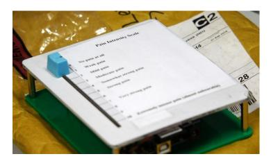
Figure 2.2. Custom built pain recording device (linear potentiometer) to record rating of pain every 2s.
