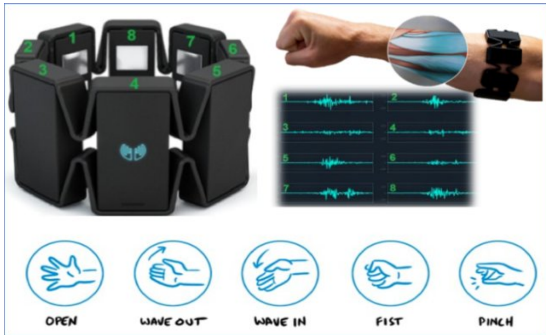
Figure 7: The illustration of Myo armband sensor by Thalmic labs, which has ceased production recently and no corresponding website is available now. The bottom panel has shown all five possible hand gestures that can be classified from built-in programs (Tatarian et al. 2018).
