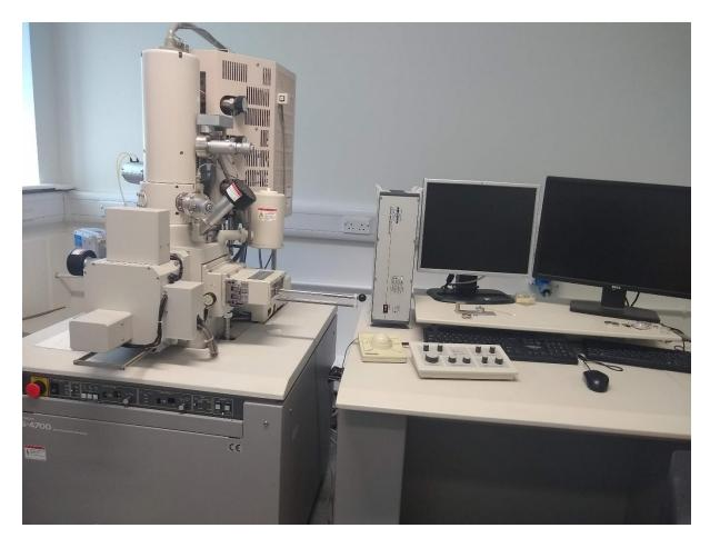
Figure 2.9. Image of the Hitachi 4700 cold field emission SEM with a Bruker X-flash Energy Dispersive X-ray Spectrometer at the University of Kent.
