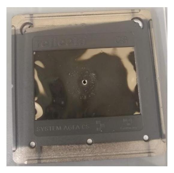
Figure 4.2. A foil that has been impacted in the photographic slide target holder. The circular area of impacts can be seem in this image.
