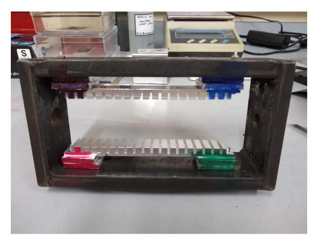
Figure 5.7. The target holder for the blast tank that was used for the LGG shots. This holder has many slots that can be used for the photographic slides at different locations.
