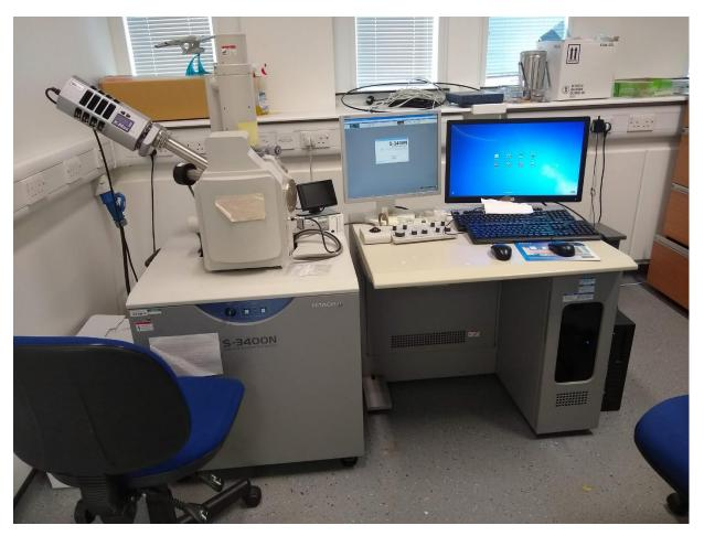
Figure 2.8. Image of the Hitachi 3400N SEM with an Oxford Instruments 80 mm2 X-max Energy Dispersive X-ray Spectrometer at the University of Kent.
