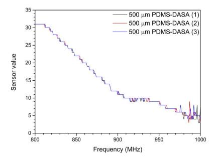
Figure 3-41 – Plots of backscattered power as sensor values, against frequency, for three runs of an RFMicron tag covered with a 500 μm-thick PDMS-DASA film (coloured).
