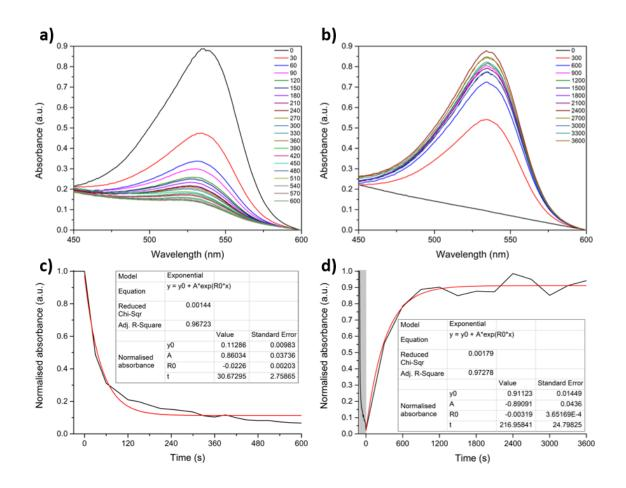
Figure 3-47 - UV-vis data acquired for AC-0.5, consisting of a) a time lapse of the forward photoswitching reaction, b) the thermal reversion, and c+d) the change in  $\lambda_{max}$  over time, for the forward and backward reactions, respectively.
