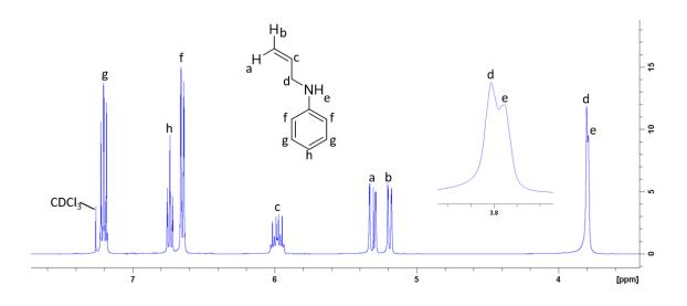
Figure 4.0-26 – <sup>1</sup>H NMR spectrum of *N*-allyl aniline, in chloroform-*d*.
