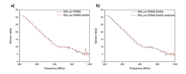
Figure 3-40 – Plots of backscattered power as sensor values, against frequency, for RFMicron tags covered with 500  $\mu$ m films of: a) PDMS and PDMS-DASA, b) PDMS-DASA open and closed.
