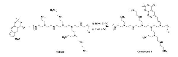
Figure 4-1 – Synthetic scheme for compound 1.
