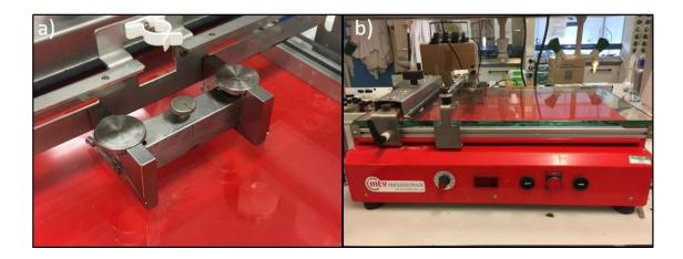
Figure 2-2 – An automatic precision film applicator CX4 from mtv messtechnik, used for the application of elastomeric films.
