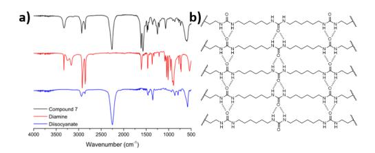
Figure 4-10 – a) FTIR spectral overlay of compound 7, hexamethylenediamine and hexamethylene diisocyanate; b) a representation of the hydrogen-bonding between polymer chains of compound 7.
