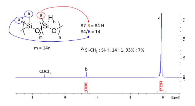
Figure 4-15 - <sup>1</sup>H NMR spectrum of poly(MHS-DMS), with calculations toward the determination of reactive Si-H sites.
