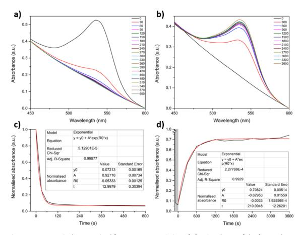
Figure 3-50 - UV-vis data acquired for SAC-0.1, consisting of a) a time lapse of the forward photoswitching reaction, b) the thermal reversion, and c+d) the change in  $\lambda_{max}$  over time, for the forward and backward reactions, respectively.
