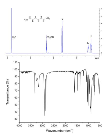
Figure 4.0-22 – <sup>1</sup>H NMR (top) and FTIR (bottom) spectra of hexamethylenediamine.
