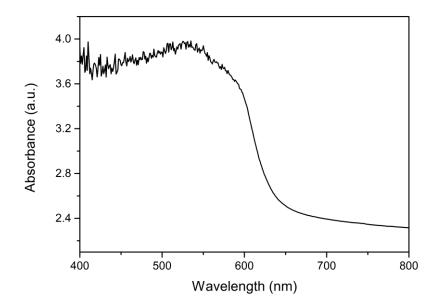
Figure 3-44 - UV-vis plot of SAC-5 after 2 hours of light irradiation.
