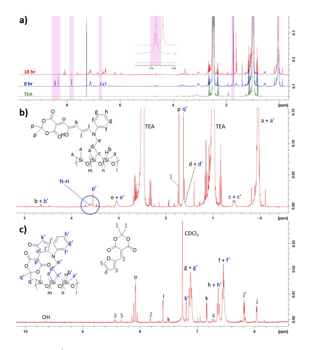
Figure 4-18 – a) <sup>1</sup>H NMR spectral overlay of TEA and the tube reaction of product 10 and MAF, at 0 and 18 hours post-TEA addition, MAF signals are highlighted by pink bands; b + c) expansions of the 18-hr <sup>1</sup>H NMR spectrum, the blue ring highlights signals potentially characteristic of unreacted amine and cyclic DASA protons (see discussion).
