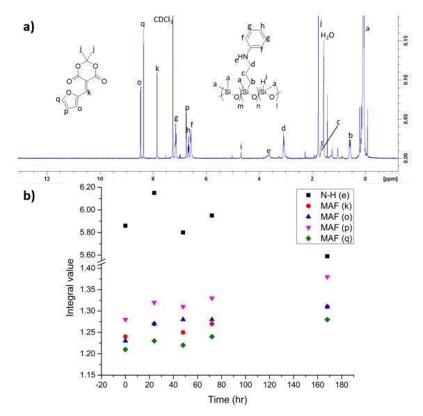
Figure 4-17 – a) <sup>1</sup>H NMR of MAF and compound 10, after 168 hrs; b) a plot of the integrals for signals e, k, o, p and q, over time.
