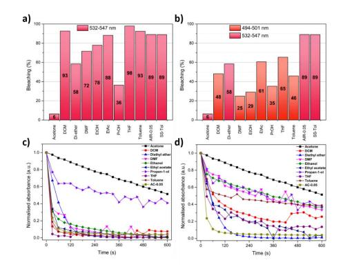
Figure 3-38 – Attained percentage photobleaching after 60 s of a) peak 1 and b) peak 2, for each swollen elastomer, a dry elastomer and the solution state (toluene). Where di-ether = diethyl ether; EtAc = ethyl acetate; PrOH = propan-1-ol. Normalised absorbance for c) peak 1 and d) peak 2, over time.
