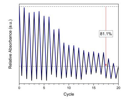
Figure 3-31 - Extension of cycling 5x15, to 20 cycles. Examination of maxima shows an overall decomposition of 81.1% of photoswitching species.
