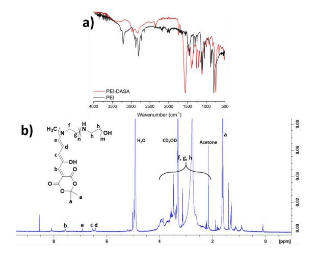
Figure 4-6 – a) FTIR of compound 4, overlaid with that of PEI 10,000; b) <sup>1</sup>H NMR of 4 in methanol- $d_4$ .
