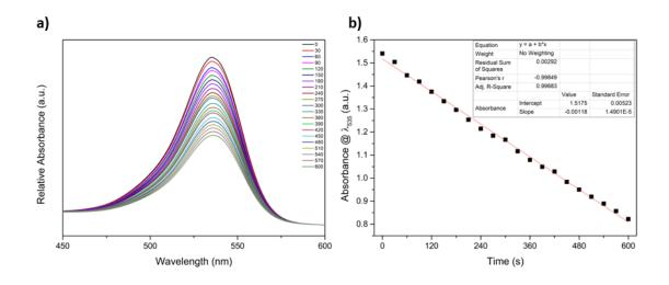
Figure 3-34 – a) UV-vis time-lapse of AC-0.05 swelled by acetone vapours, b) the absorbance values of  $\lambda_{max}$  = 535 nm, during each 30-second period.
