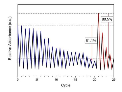
Figure 3-32 - The 5x15 study further extended by 5 cycles, to include oven-reversion steps of 10 minutes.
