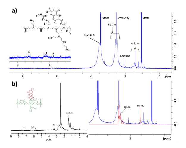
Figure 4-2 – a) <sup>1</sup>H NMR spectrum of compound 1, in DMSO- $d_6$ ; b) <sup>1</sup>H NMR spectra of a previously-reported PEI-DASA example (left)<sup>25</sup> and compound 1 overlaid with PEI-600 (right).
