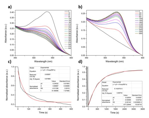
Figure 3-52 - UV-vis data acquired for SAC-1, consisting of a) a time lapse of the forward photoswitching reaction, b) the thermal reversion, and c+d) the change in  $\lambda_{max}$  over time, for the forward and backward reactions, respectively.
