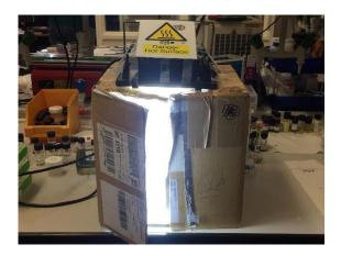
Figure 3-4 - A custom-made light irradiation box; a 50 W, 6500 K full spectrum LED floodlight attached to a cardboard box lined with reflective foil sheets.
