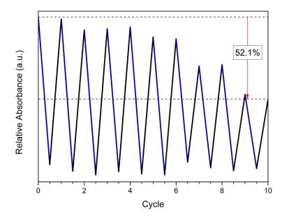
Figure 3-29 - UV-vis cycling study of AC-0.05, showing a 52.1 % decrease in absorbance postoven reversion, within 10 cycles. Cycles constituted a 15-minute light exposure step, followed by a 5-minute oven-reversion period – designated '5x15'.
