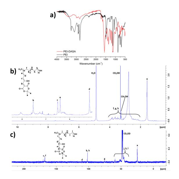
Figure 4-7 – a) FTIR of compound 5, overlaid with that of PEI 2,500; b) <sup>1</sup>H NMR of 5 in methanol $d_4$ ; c) <sup>13</sup>C NMR of 5 in methanol- $d_4$ .
