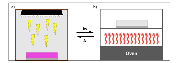
Figure 3-21 - Graphic representation of photoswitching (left) and oven-reversion (right). The photoswitching consists of placing the sample inside a cardboard box which has an LED lamp attached to the ceiling.
