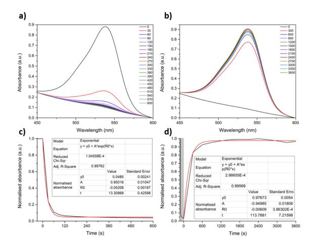
Figure 3-45 - UV-vis data acquired for AC-0.05, consisting of a) a time lapse of the forward photoswitching reaction, b) the thermal reversion, and c+d) the change in  $\lambda_{max}$  over time, for the forward and backward reactions, respectively.
