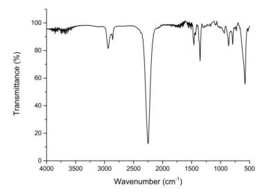
Figure 4.0-21 – FTIR spectrum of hexamethylene diisocyanate.
