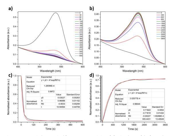
Figure 3-49 - UV-vis data acquired for SAC-0.05, consisting of a) a time lapse of the forward photoswitching reaction, b) the thermal reversion, and c+d) the change in  $\lambda_{max}$  over time, for the forward and backward reactions, respectively.
