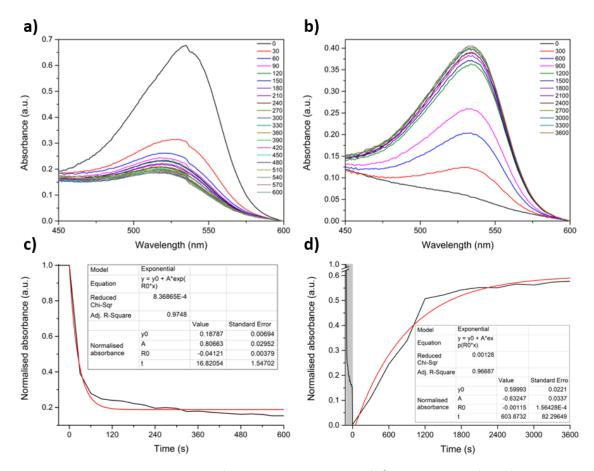
Figure 3-51 - UV-vis data acquired for SAC-0.5, consisting of a) a time lapse of the forward photoswitching reaction, b) the thermal reversion, and c+d) the change in  $\lambda_{max}$  over time, for the forward and backward reactions, respectively.
