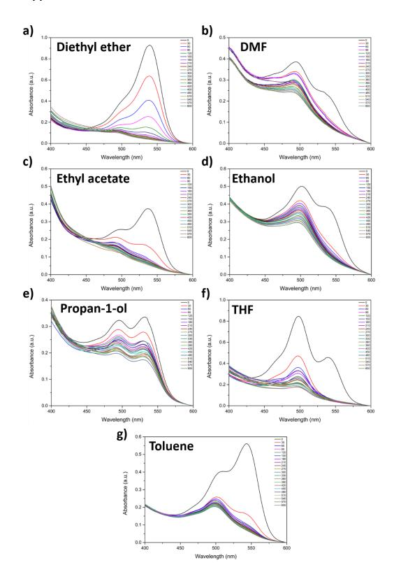
Figure 3-53 – UV-vis time-lapse data for AC-0.05 elastomer swollen by: a) diethyl ether, b) DMF, c) ethyl acetate, d) ethanol, e) propan-1-ol, f) THF, g) toluene.
