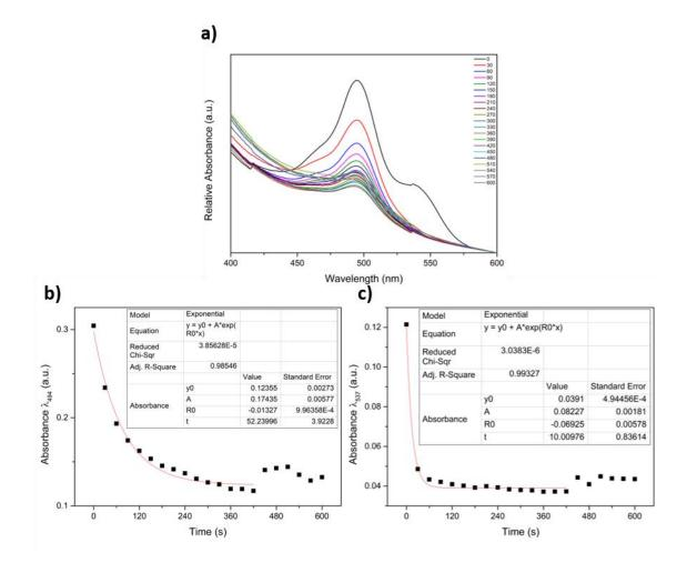
Figure 3-35 - a) UV-vis time-lapse of AC-0.05 swelled by DCM vapours – note the large baseline drift, b) the absorbance values of  $\lambda_{max}$  = 494 nm, during each 30-second period, c) the absorbance values of  $\lambda_{max}$  = 537 nm, during each 30-second period.
