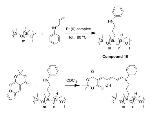
Figure 4-14 – Synthetic schemes toward the production of a DASA-functionalised polysiloxane backbone.
