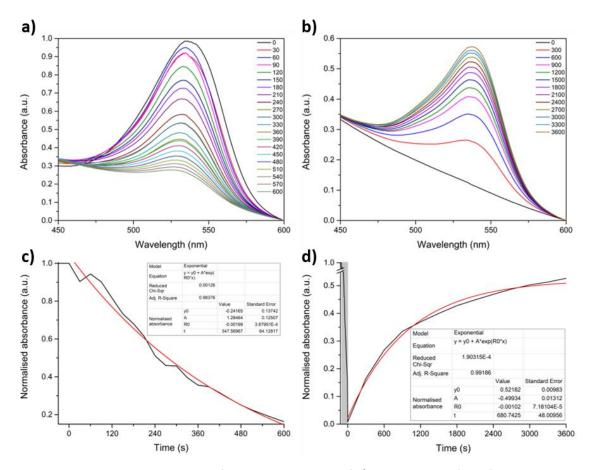
Figure 3-48 - UV-vis data acquired for AC-1, consisting of a) a time lapse of the forward photoswitching reaction, b) the thermal reversion, and c+d) the change in  $\lambda_{max}$  over time, for the forward and backward reactions, respectively.
