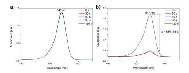
Figure 3-37 – UV-vis spectra over time, during white light irradiation of HexDASA in: a) DCM and b) toluene.
