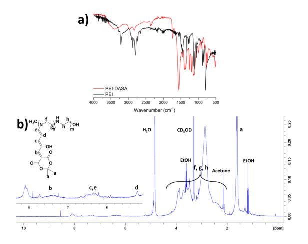
Figure 4-5 – a) FTIR of compound 3a, overlaid with that of PEI 10,000; b) <sup>1</sup>H NMR of 3b in methanol- $d_4$ .
