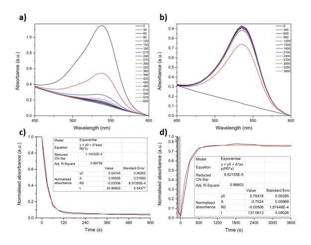
Figure 3-46 - UV-vis data acquired for AC-0.1, consisting of a) a time lapse of the forward photoswitching reaction, b) the thermal reversion, and c+d) the change in  $\lambda_{max}$  over time, for the forward and backward reactions, respectively.
