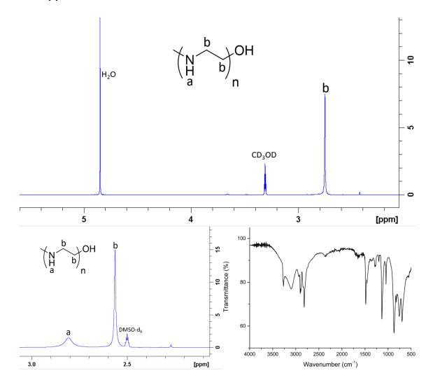
Figure 4.0-20 – <sup>1</sup>H NMR of PEI 2,500 in methanol- $d_4$  (top) and DMSO- $d_6$  (bottom, left), alongside its FTIR spectrum (bottom, right).
