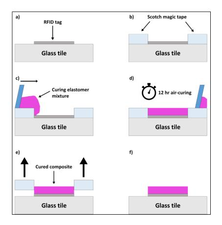
**Figure 3-39** – A modified diagrammatic representation of film-casting, using the Scotch tape-well method:<sup>107</sup> a + b) A UHF RFID tag is taped to a glass substrate using Scotch magic tape; c + d) the speed-mixed elastomer mixture is applied using a doctor blade and allowed to air-cure overnight, in a dark environment; e) removal of tape; f) finished product.
