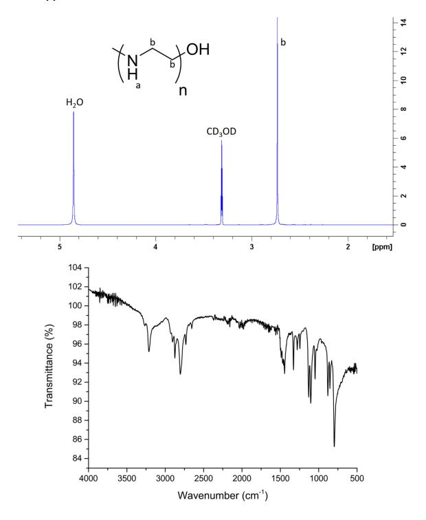
Figure 4.0-19 - <sup>1</sup>H NMR of PEI 10,000 in methanol-d<sub>4</sub> (top) and its FTIR spectrum (bottom, right).
