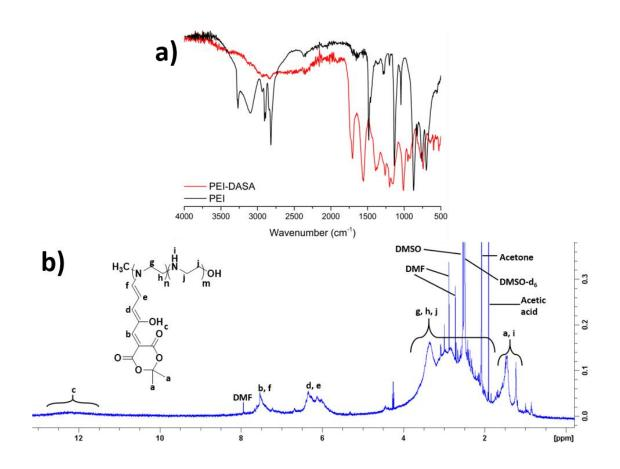
Figure 4-8 – a) FTIR of compound 6, overlaid with that of PEI 2,500; b) <sup>1</sup>H NMR of 6 in DMSO $d_6$
