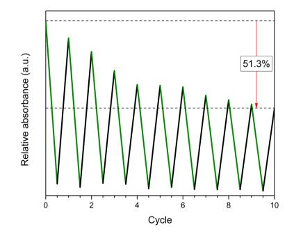
Figure 3-28 - UV-vis cycling study of AC-0.05, showing a 51.3 % decrease in absorbance postoven reversion, within 10 cycles. Cycles constituted a 5-minute light exposure step, followed by a 5-minute oven-reversion period – designated '5x5'.
