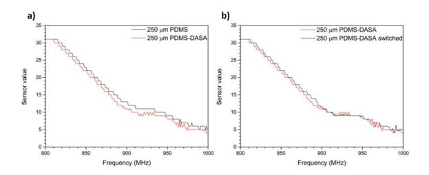
Figure 3-42 - Plots of backscattered power as sensor values, against frequency, for RFMicron tags covered with 250 μm films of: a) PDMS, b) PDMS-DASA.
