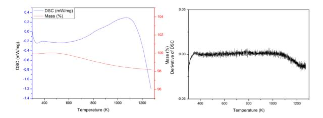
Figure A3.76: TGA/DSC results  $Bi_{0.15}Na_{0.85}Fe_{0.15}Nb_{0.85}O_3$  (a) Full TGA/DSC plot from 298 K to 1270 K, (b) Derivative of DSC against temperature from 298 K to 1270 K.
