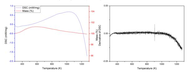
Figure A3.69: TGA/DSC results for  $Bi_{0.8}Na_{0.2}Fe_{0.8}Nb_{0.2}O_3$  (a) Full TGA/DSC plot from 298 K to 1270 K, (b) Derivative of DSC against temperature from 298 K to 1270 K.
