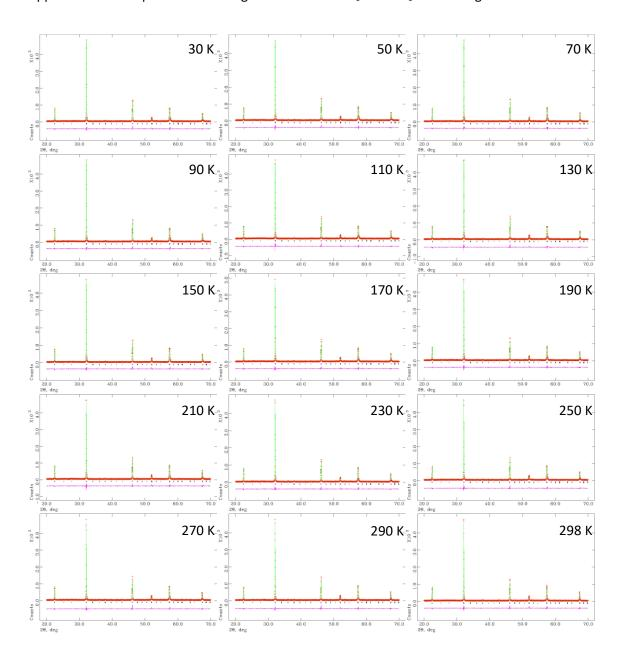
**Figure A3.63:** Rietveld refinements obtained from LT PXRD of  $Bi_{0.2}Na_{0.8}Fe_{0.2}Nb_{0.8}O_3$  in the temperature ranges 30 K to 298 K.
