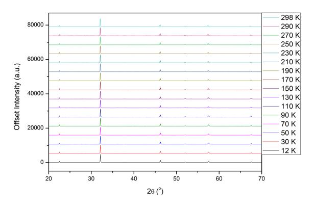
**Figure A3.60:** All patterns for the LT PXRD of  $Bi_{0.2}Na_{0.8}Fe_{0.2}Nb_{0.8}O_3$ . 12K pattern intensity has been scaled down to match the intensities of the other temperature points that were taken with shorter scan times.
