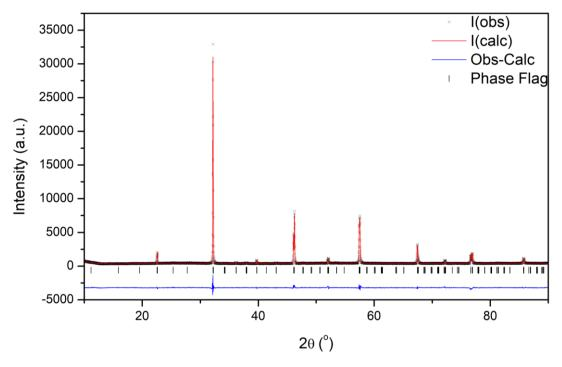
**Figure A3.53:** Rietveld refinement of 12 K PXRD data collected for  $Bi_{0.3}Na_{0.7}Fe_{0.3}Nb_{0.7}O_3$ ;  $\chi^2 = 2.213$ ,  $R_{wp} = 6.63\%$  and  $R_p = 5.07$ ; the black crosses represent the observed intensity, the red line represents the calculated intensity from the model, the blue line represents the difference between the observed pattern and calculated pattern and the black tick marker represents the  $P2_1$ ma model.
