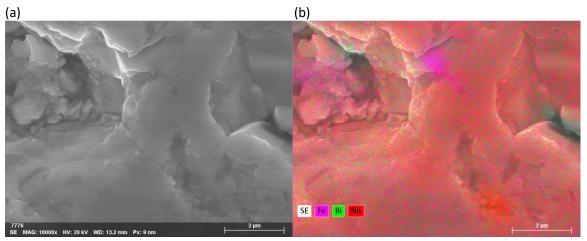
**Figure 3.24:** Scanning Electron microscopy images collected for a polished Bi<sub>0.9</sub>Na<sub>0.1</sub>Fe<sub>0.9</sub>Nb<sub>0.1</sub>O<sub>3</sub> pellet. (a) Secondary electron image and (b) Electron Dispersive X-Ray Analysis map.
