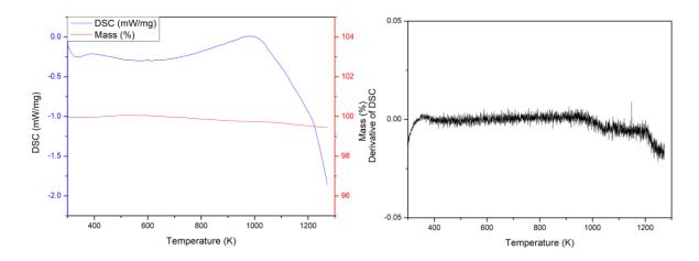
Figure A3.73: TGA/DSC results for  $Bi_{0.325}Na_{0.675}Fe_{0.325}Nb_{0.675}O_3$  (a) Full TGA/DSC plot from 298 K to 1270 K, (b) Derivative of DSC against temperature from 298 K to 1270 K.
