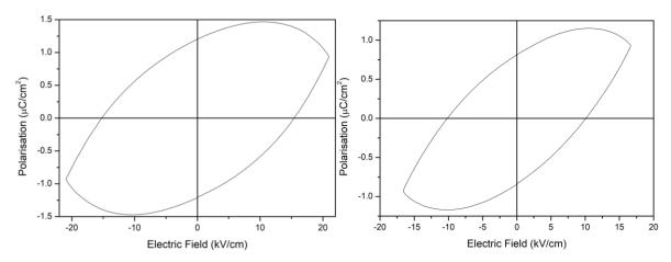
**Figure 4.33:** PE loop data collected for Bi<sub>0.5</sub>Na<sub>0.5</sub>Fe<sub>0.5</sub>Nb<sub>0.5</sub>O<sub>3</sub>, (a) Hysteresis loop for pure sample Frequency: 20 Hz and Amplitude: 3000 V and (b) Hysteresis loop for sample modified with 2% PVB binder and 0.2% MnO₂ Frequency: 10 Hz and Amplitude: 2000 V.
