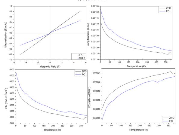
**Figure A3.82:** Magnetic data from SQUID for  $Bi_{0.7}Na_{0.3}Fe_{0.7}Nb_{0.3}O_3$ , (a) Hysteresis loops from 2 K to 300 K at fields from 5 T to 5 T, (b) Variable temperature Zero field cooled and Field cooled data at 0.1, (c)  $\chi$  SQUID data, (d)  $1/\chi$  SQUID data.
