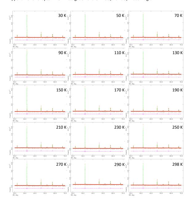
**Figure A3.58:** Rietveld refinements obtained from LT PXRD of  $Bi_{0.25}Na_{0.75}Fe_{0.25}Nb_{0.75}O_3$  in the temperature ranges 30 K to 298 K.
