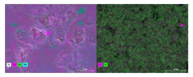
**Figure A1.16:** Scanning Electron microscopy images of  $Bi_{0.9}Na_{0.1}Fe_{0.9}Nb_{0.1}O_3$  pellet. Electron Dispersive X-Ray Analysis map.
