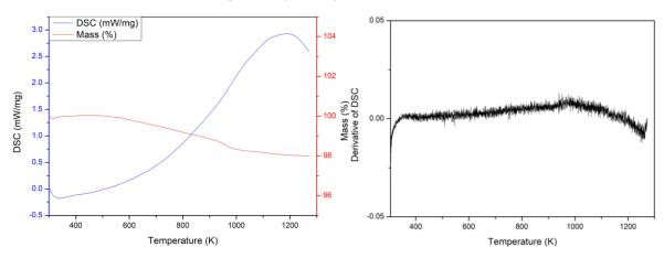
Figure A3.77: TGA/DSC results  $Bi_{0.05}Na_{0.95}Fe_{0.05}Nb_{0.95}O_3$  (a) Full TGA/DSC plot from 298 K to 1270 K, (b) Derivative of DSC against temperature from 298 K to 1270 K.
