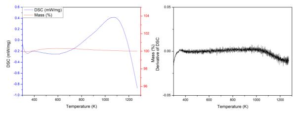
Figure A3.75: TGA/DSC results  $Bi_{0.2}Na_{0.8}Fe_{0.2}Nb_{0.8}O_3$  (a) Full TGA/DSC plot from 298 K to 1270 K, (b) Derivative of DSC against temperature from 298 K to 1270 K.
