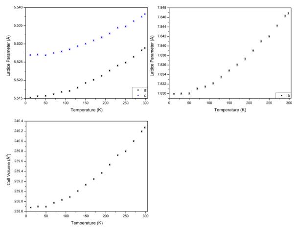
**Figure A3.62:** LT PXRD of  $Bi_{0.2}Na_{0.8}Fe_{0.2}Nb_{0.8}O_3$ : (a) + (b) Lattice Parameter against temperature plot, (c) Cell Volume against temperature plot.
