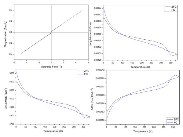
**Figure A3.80:** Magnetic data from SQUID for  $Bi_{0.8}Na_{0.2}Fe_{0.8}Nb_{0.2}O_3$ , (a) Hysteresis loops from 2 K to 300 K at fields from 5 T to 5 T, (b) Variable temperature Zero field cooled and Field cooled data at 0.1, (c)  $\chi$  SQUID data, (d)  $1/\chi$  SQUID data.
