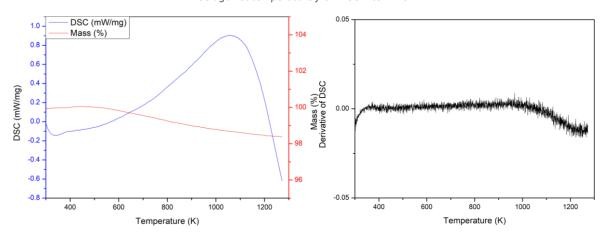
Figure A3.72: TGA/DSC results for  $Bi_{0.35}$ Na $_{0.65}$ Fe $_{0.35}$ Nb $_{0.65}$ O $_3$  (a) Full TGA/DSC plot from 298 K to 1270 K, (b) Derivative of DSC against temperature from 298 K to 1270 K.
