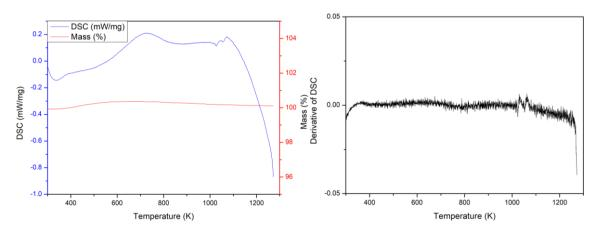
Figure A3.67: TGA/DSC results for  $Bi_{0.925}Na_{0.075}Fe_{0.925}Nb_{0.075}O_3$  (a) Full TGA/DSC plot from 298 K to 1270 K, (b) Derivative of DSC against temperature from 298 K to 1270 K.
