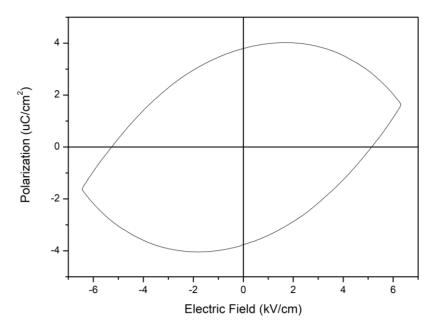
Figure 3.25: PE loop data collected for  $Bi_{0.9}Na_{0.1}Fe_{0.9}Nb_{0.1}O_3$ , material modified with 2% PVB binder and 0.2%  $TiO_2$  Frequency: 10 Hz and Amplitude: 800 V.
