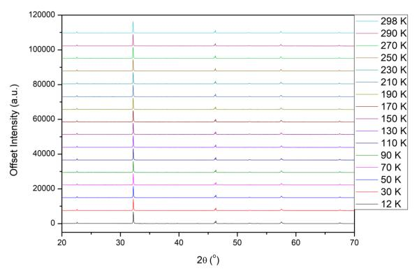
**Figure A3.56:** All patterns for the LT PXRD of  $Bi_{0.25}Na_{0.75}Fe_{0.25}Nb_{0.75}O_3$ . 12K pattern intensity has been scaled down to match the intensities of the other temperature points that were taken with shorter scan times.
