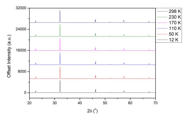
**Figure A3.59:** Selection of patterns for the LT PXRD of  $Bi_{0.2}Na_{0.8}Fe_{0.2}Nb_{0.8}O_3$ . 12K pattern intensity has been scaled down to match the intensities of the other temperature points that were taken with shorter scan times.
