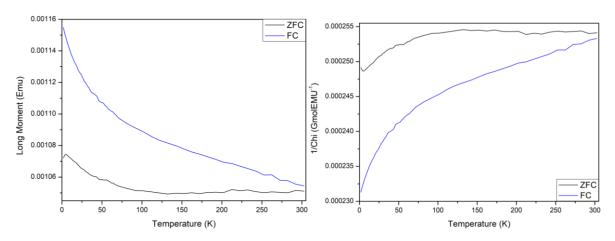
**Figure A3.79:** Magnetic data from SQUID for  $Bi_{0.85}Na_{0.15}Fe_{0.85}Nb_{0.15}O_3$ , (a) Zero field cooled and Field cooled data at 0.1 T, (b)  $1/\chi$  SQUID data.
