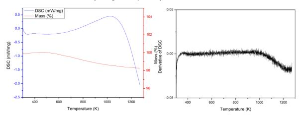
**Figure A3.74:** TGA/DSC results Bi<sub>0.3</sub>Na<sub>0.7</sub>Fe<sub>0.3</sub>Nb<sub>0.7</sub>O<sub>3</sub> (a) Full TGA/DSC plot from 298 K to 1270 K, (b) Derivative of DSC against temperature from 298 K to 1270 K.
