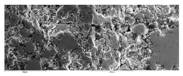
**Figure A1.17:** Scanning Electron microscopy Secondary electron images of  $Bi_{0.9}Na_{0.1}Fe_{0.9}Nb_{0.1}O_3$  pellet
