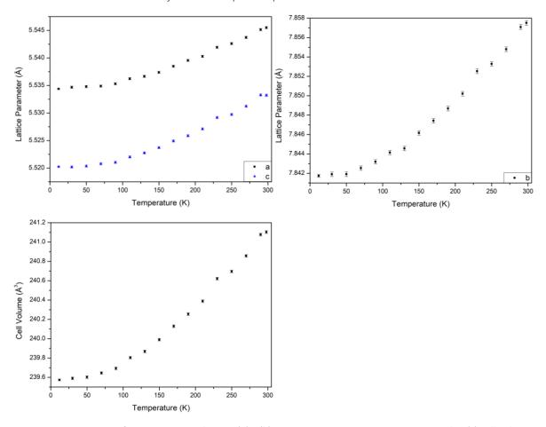
**Figure A3.57:** LT PXRD of  $Bi_{0.25}Na_{0.75}Fe_{0.25}Nb_{0.75}O_3$ : (a) + (b) Lattice Parameter against temperature plot, (c) Cell Volume against temperature plot.
