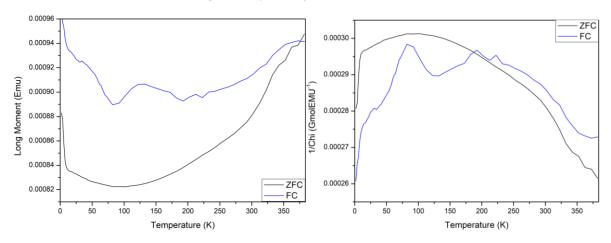
**Figure A3.78:** Magnetic data from SQUID for  $Bi_{0.95}Na_{0.05}Fe_{0.95}Nb_{0.05}O_3$ , (a) Zero field cooled and Field cooled data at 0.1 T, (b)  $1/\chi$  SQUID data.
