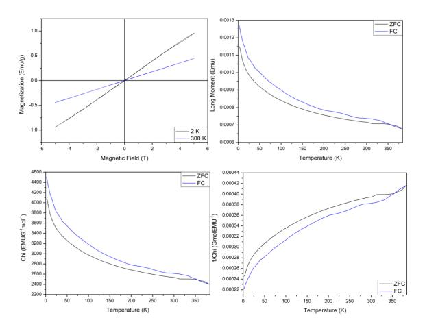
Figure A3.83: Magnetic data from SQUID for  $Bi_{0.65}Na_{0.35}Fe_{0.65}Nb_{0.35}O_3$ , (a) Hysteresis loops from 2 K to 300 K at fields from -5 T to 5 T, (b) Variable temperature Zero field cooled and Field cooled data at 0.1, (c)  $\chi$  SQUID data, (d)  $1/\chi$  SQUID data.
