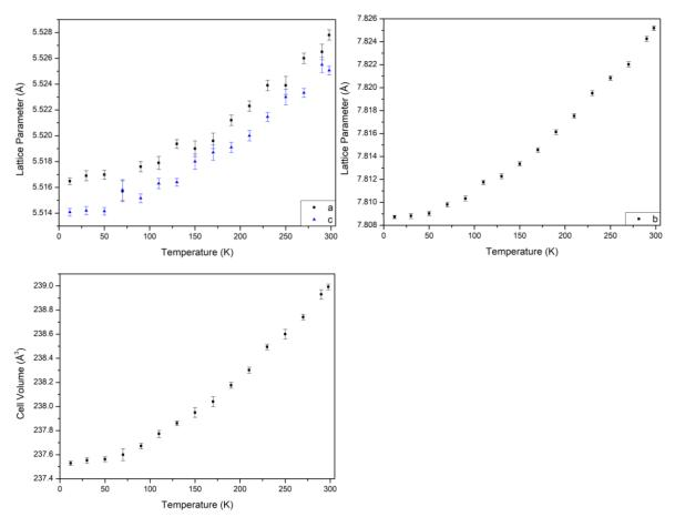
**Figure A3.65:** LT PXRD of  $Bi_{0.1}Na_{0.9}Fe_{0.1}Nb_{0.9}O_3$ : (a) + (b) Lattice Parameter against temperature plot, (c) Cell Volume against temperature plot.
