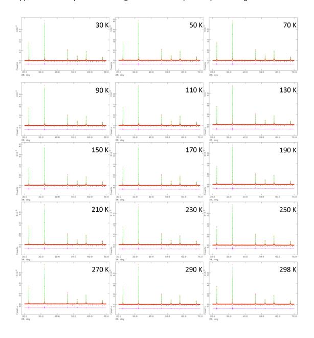
Figure A3.66: Rietveld refinements obtained from LT PXRD of  $Bi_{0.1}Na_{0.9}Fe_{0.1}Nb_{0.9}O_3$  in the temperature ranges 30 K to 298 K.
