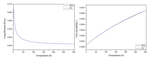
**Figure A3.86:** Magnetic data from SQUID for  $Bi_{0.2}Na_{0.8}Fe_{0.2}Nb_{0.8}O_3$ , (a) Zero field cooled and Field cooled data at 0.1 T, (b)  $1/\chi$  SQUID data.
