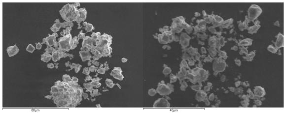
$\textbf{\textit{Figure A1.18:} Scanning Electron Secondary electron microscopy images of Bi}_{0.9} Na_{0.1} Fe_{0.9} Nb_{0.1} O_3 powder.$
