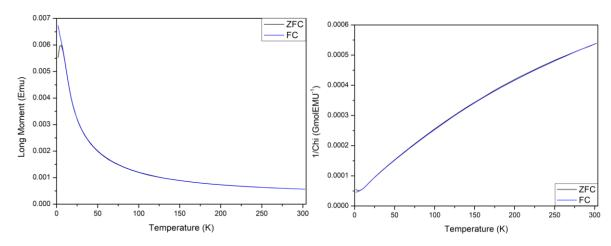
**Figure A3.85:** Magnetic data from SQUID for  $Bi_{0.3}Na_{0.7}Fe_{0.3}Nb_{0.7}O_3$ , (a) Zero field cooled and Field cooled data at 0.1 T, (b)  $1/\chi$  SQUID data.
