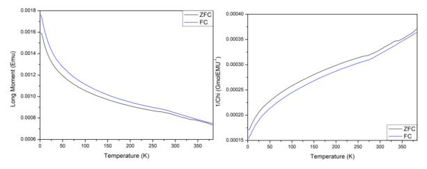
**Figure A3.84:** Magnetic data from SQUID for  $Bi_{0.6}Na_{0.4}Fe_{0.6}Nb_{0.4}O_3$ , (a) Zero field cooled and Field cooled data at 0.1 T, (b)  $1/\chi$  SQUID data.
