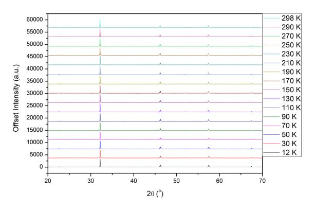
**Figure A3.52:** All patterns for the LT PXRD of  $Bi_{0.3}Na_{0.7}Fe_{0.3}Nb_{0.7}O_3$ . 12K pattern intensity has been scaled down to match the intensities of the other temperature points that were taken with shorter scan times.
