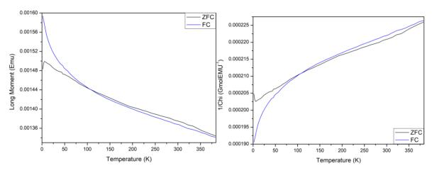
**Figure A3.81:** Magnetic data from SQUID for  $Bi_{0.75}Na_{0.25}Fe_{0.75}Nb_{0.25}O_3$ , (a) Zero field cooled and Field cooled data at 0.1 T, (b)  $1/\chi$  SQUID data.
