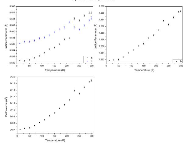
**Figure A3.54:** LT PXRD of  $Bi_{0.3}Na_{0.7}Fe_{0.3}Nb_{0.7}O_3$ : (a) + (b) Lattice Parameter against temperature plot, (c) Cell Volume against temperature plot.
