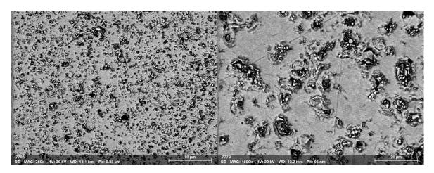
**Figure A1.15:** Scanning Electron microscopy back scattered electron images of  $Bi_{0.9}Na_{0.1}Fe_{0.9}Nb_{0.1}O_3$  pellet.
