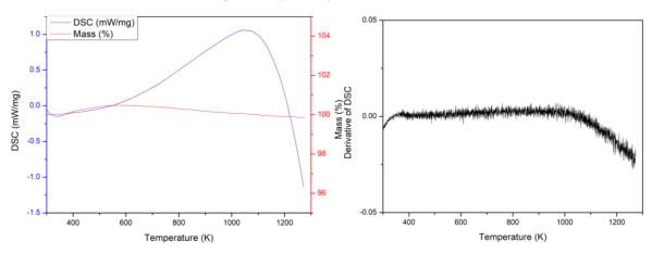
**Figure A3.71:** TGA/DSC results for  $Bi_{0.65}Na_{0.35}Fe_{0.65}Nb_{0.35}O_3$  (a) Full TGA/DSC plot from 298 K to 1270 K, (b) Derivative of DSC against temperature from 298 K to 1270 K.
