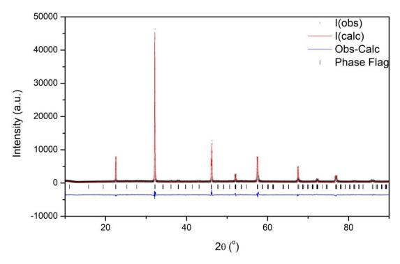
**Figure A3.61:** Rietveld refinement of 12 K PXRD data collected for  $Bi_{0.2}Na_{0.8}Fe_{0.2}Nb_{0.8}O_3$ ;  $\chi^2 = 4.642$ ,  $R_{wp} = 8.78\%$  and  $R_p = 6.31$ ; the black crosses represent the observed intensity, the red line represents the calculated intensity from the model, the blue line represents the difference between the observed pattern and calculated pattern and the black tick marker represents the  $P2_1ma$  model.
