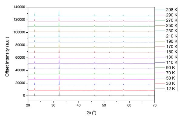
**Figure A3.64:** All patterns for the LT PXRD of  $Bi_{0.1}Na_{0.9}Fe_{0.1}Nb_{0.9}O_3$ . 12K pattern intensity has been scaled down to match the intensities of the other temperature points that were taken with shorter scan times.
