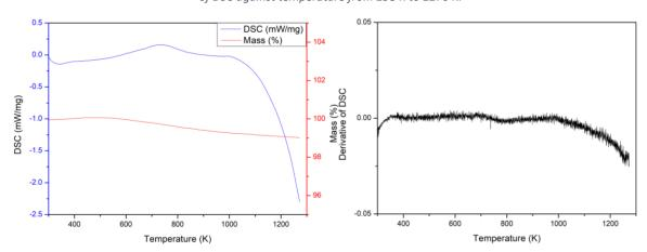
Figure A3.68: TGA/DSC results for  $Bi_{0.875}Na_{0.125}Fe_{0.875}Nb_{0.125}O_3$  (a) Full TGA/DSC plot from 298 K to 1270 K, (b) Derivative of DSC against temperature from 298 K to 1270 K.
