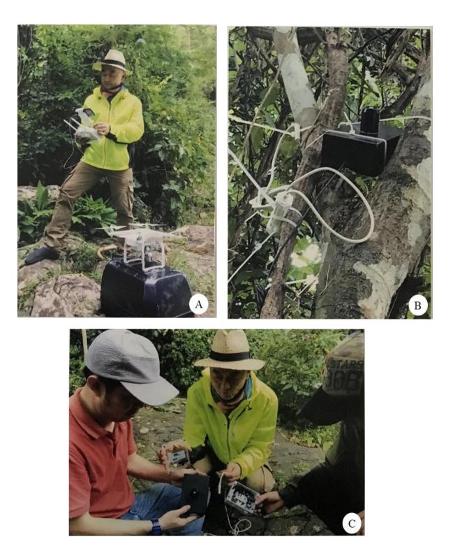
**Appendices Figures 10** (A-C) Preparing to set up the Hobo Data logger onto the tree trunk in order to measure the moisture, relative humidity, and temperature for fourteen days.
