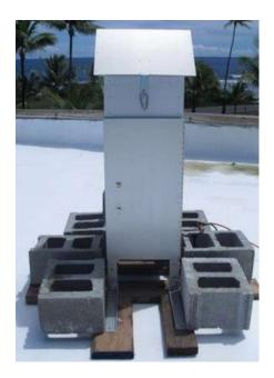
Figure 3.1: The Kwajalein micrometeorite collector in position on the Kwajalein atoll. The breeze blocks are to hold the collector in position.
