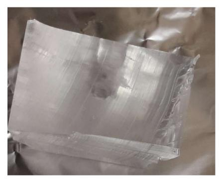
Figure 6.5: The STST projectile having been captured in the silicone rubber. The projectile travelled straight into the target without any evidence of direction change, or impacts into the EVT itself.
