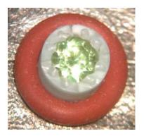
**Figure 6.11**: Photograph of the olivine projectile positioned inside of the quartered sabot prior to loading in the launch tube
