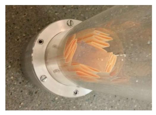
Figure 6.1: The loaded capture medium cartridge (Mylar walled) in the EVT.
