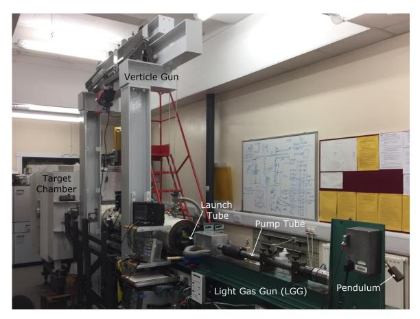
Figure 3.5: The LGG facility at the University of Kent as of November 2017
