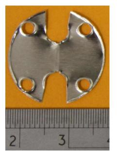
Figure 3.34: An electronic burst disk foil layer with the notches cut (scale divisions are 0.5 mm).
