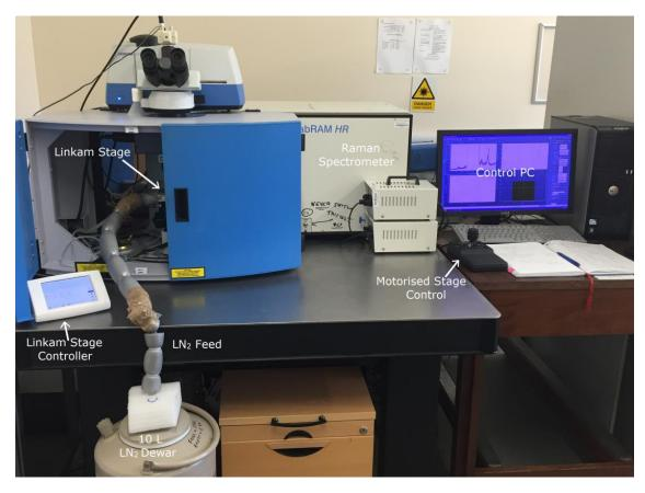
Figure 4.12: The Raman spectrometer configured for a low temperature experiment.
