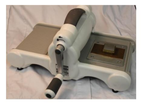
Figure 3.23: The prototype punch being used to punch a 100 micron thick aluminium foil electronic burst disk on a "Sizzex Big Shot" die cutting machine.
