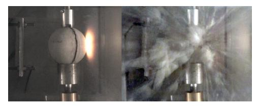
Figure 3.8: (left) A spherical target in the rotating target holder at the moment of impact and (Right) during complete disruption of the target (approximately 5 milliseconds later).
