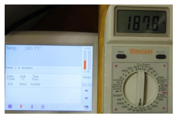
Figure 4.15: An example picture of the Linkam stage controller showing the stage temperature and the multimeter showing the resistance of the PT100 sensor.
