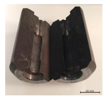
Figure 3.12: A central breech that has been split in two after being impacted by a piston at too great a velocity.
