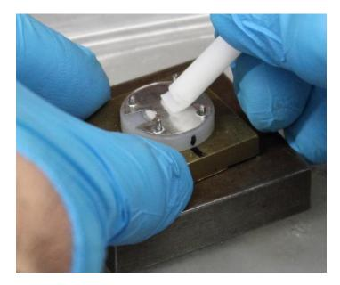
Figure 3.38: The smoothing tool being used on the surface of the foil attached to the burst disk support.
